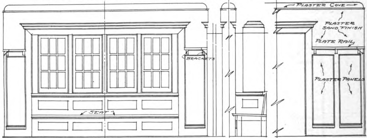
DINING ROOM TRIM, SEAT PLATE RAIL, AND PANELING
