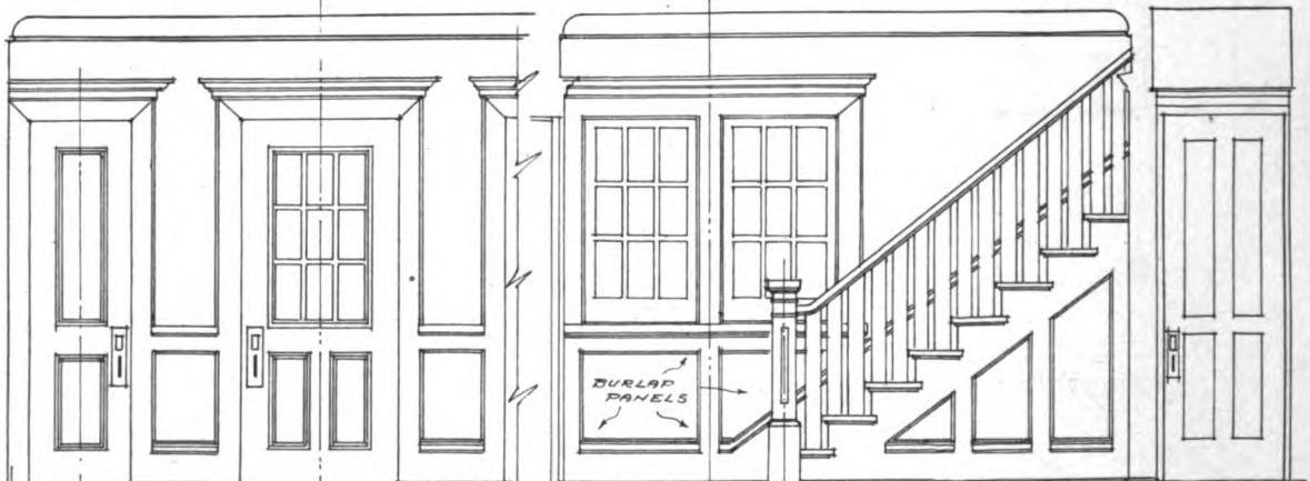
HALL ENTRY AND CLOSET DOORS, STAIR DETAILS
