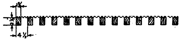
Fig. 2—Side View of the Mat System
