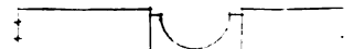
Cove Mouldings of Front and Closet Door Trim—Scale 3 In. to the Foot
