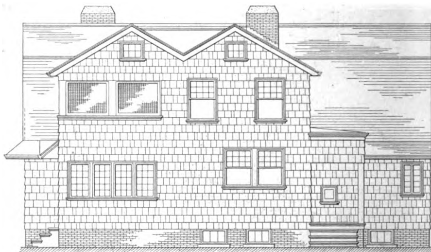
Rear Elevation of the House, Showing Sleeping Porch on Second Floor—Scale 3/32 In. to the Foot
