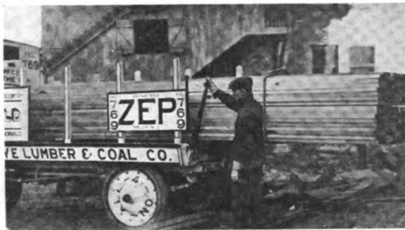
Fig. 4—The First Operation in Unloading the Truck Is Releasing the Pawl to Work the Lever
