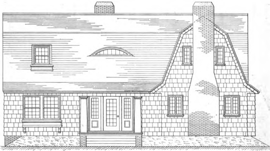
Front Elevation, Showing Recessed Entrance and Outside Chimney—Scale 3/32 In. to the Foot
