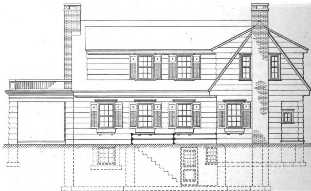
Rear Elevation of the House, Showing the Area Stairs to the Basement—Scale 3/32 In. to the Foot
