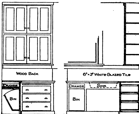
Elevation of Kitchen Case with Section Through Flour Bin—Scale 1/4 In. to the Foot
