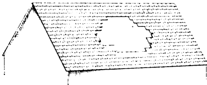
FIG. 4—BROKEN SLATE REMOVED FOR REPAIRS
