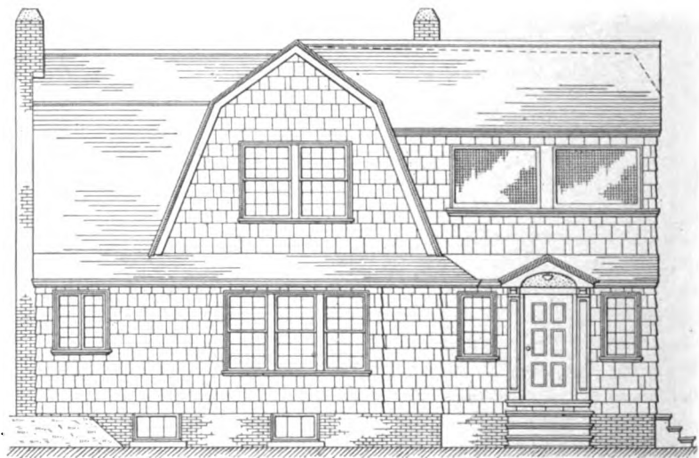
Right Side Elevation Showing Outside Door to Library—Scale 3/32 In. to the Foot
