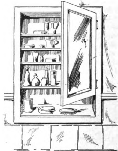
Fig. 5—Toilet Cabinet in Bathroom Wall
