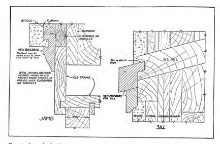
Practical method of treating window frames in overcoating old houses when siding or shingles are not removed
