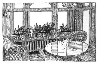
Fig. 9. Wide shelves over a radiator serve to reduce efficiency about 5 per cent.
