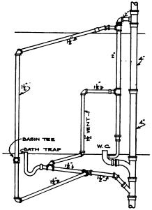
Arrangement of vent and waste pipes for bathroom number two
