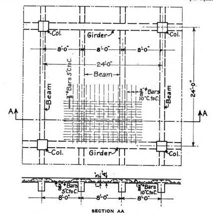
Fig. 6. Plan of interior bay above, with section on line A A below
