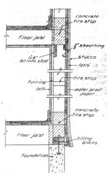
Section showing fire stopping and general features of stucco construction.
