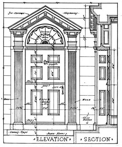
Fig. 4.—Measured drawing of Dutch door.
