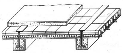
Fig. 85—When light floors with deep beams are necessary, this type of construction is good
