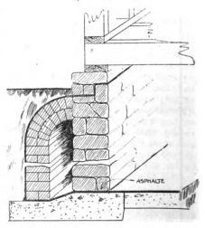
Fig. 3—A type of wall construction where conditions are severe
