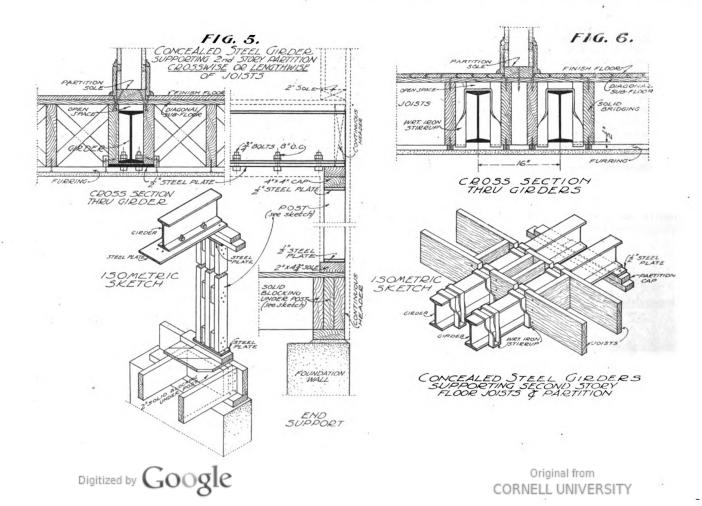
about ½-in. to the foot. Therefore, in any case, as well as this one, the distance from the underside of the sub-floor to the top of the steel girder should never be less than 1/24th the distance from the underside of the floor to the bottom, or bearing surface, of the joist-plate.
