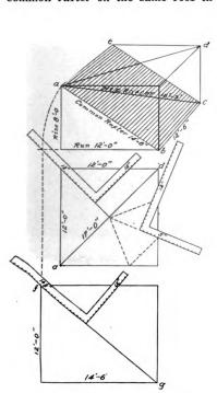
Fig. 38—Illustrating how to find octagon jack cuts
