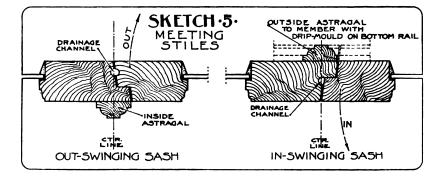
top rail, and they must be so located as not to be in line with the screws that fasten the hinges in place. By plowing the channels close to the exterior face of the sash and then hanging the sash on "parliament" butts, the channels will be left unobstructed. In any case, the lip on the bottom rail of the out-swinging sash should be far enough back to allow of the side channels draining directly onto the sill, as indicated in the sketch.
