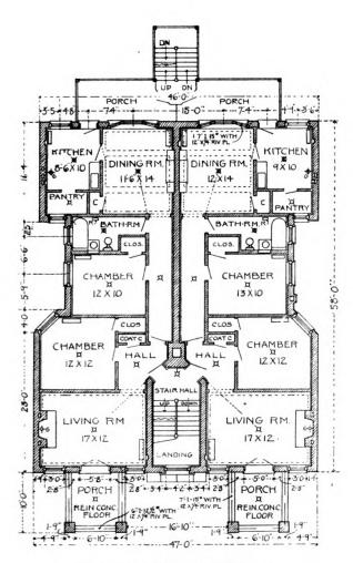
Typical floor plan, scale 1/16" = 1'
