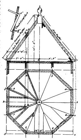
Fig. 35--How to proceed when getting cuts of rafters on an octagon roof
