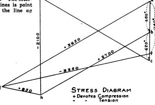
Fig. 3. Diagram of stresses in trues
