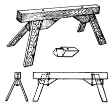
Construction of a type of saw-buck that is an efficient aid to the contractor
