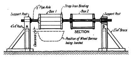
A tip box that helps to eliminate waste in measuring materials for concrete
