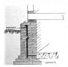
Fig. 4—A double wall provides an air space
