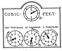
Fig. 1 and 2-Showing the usual arrangement of dials on a gas meter
