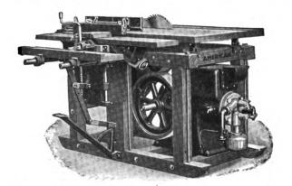
"American" Contractors' Variety Woodworker with Gas oline Engine Built In; Also Made with Self-Contained Electric Motor or for Belt Drive
