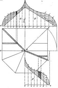
Fig. 39—Showing the proper method of getting cuts on an ogee roof
