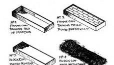
Progress sketches illustrating various steps in constructing the blocks
