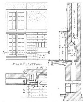
Elevations and sections, scale 1/16 in. = 1 ft., showing how to construct a fireplace.
