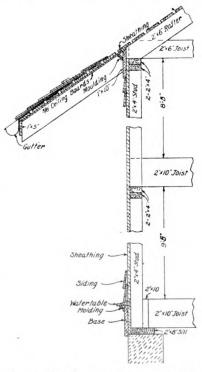
Fig. 3-T-Sill and cornice construction
