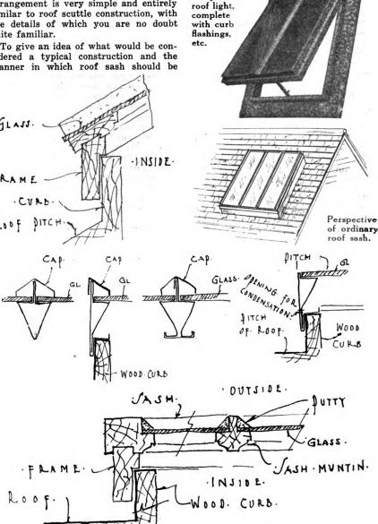
Details Showing How to Construct Weather-Tight Roof Sash
