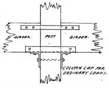
Fig. 1—A column cap made up of ordinary structural shapes
