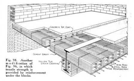
is carried on hollow-tile girder coverings supported by the lower flange of the steel girder.
