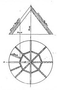
Fig. 36—Getting cuts for a round roof
