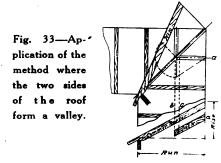
point (u) where the line (t) (u) crosses the rum of the second jack on the narrow side over to (H), where the rim of jack strikes the rim of hip  $(u)^{\bullet}(H)$ , is the exact measurement for jacks on the short side of the roof. The measurement for the jacks on the other side can be found in the same way.
