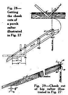
jack can be used as a measure for laying off the other jacks on the same side.
