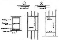
Determining spacing of studs
