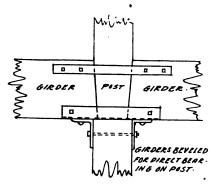
Fig. 2—Construction when it is necessary for girders to bear directly on the post
