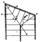
Fig. 34 — Illustrating how to determine where ridge pole and upper ends of hips will meet when end of roof is out of square
