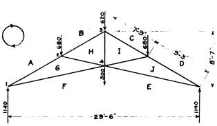
Fig. 2. Diagram of truss, showing calculation of loads
