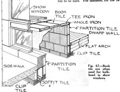
in. long the T beams should be spaced 19 in, on centers.
