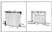
Fig. 1. Shelves over a radiator reduce efficiency
