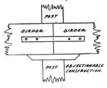
Fig. 4—A common form of construction which is not good. No tie is provided between post and girders, which might prove disastrous in case of settlement due to insufficient footing or shock
