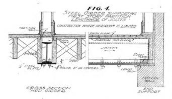
the case may be. The solid bridging, besides stiffening the floor-joists and distributing load to the girder, effectively also stops the spread of fire. But it must always be put in with the grain horizontal, so as to shrink the same amount, vertically, as the joists themselves.
