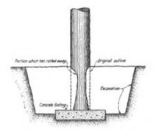
Fig. 1. Condition of the post to be repaired
