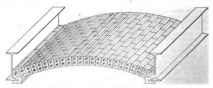
Fig. 91. A single rowlock arch made of hollow brick, which is very similar to one laid up of hollow tileriginal from
