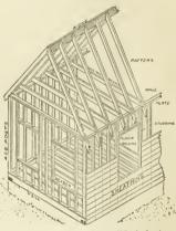
Fig. 4-Bungalow Frame Which Lacks Required Bracing
