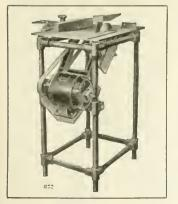
An excellent apping gauge is provided which ones 8½ inches from the saw and held in any position by a quick actor clamp. It is adjustable for align one with saw and can be removed quickly for long cut-off work.
