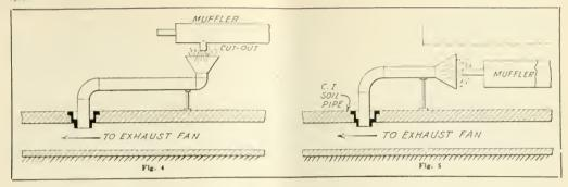
As this vapor is heavier than air, it falls to the floor and will flow out of an opening of this kind like water, unless opposed by too strong a wind pressure. When the weather is warm enough, open doors provide the best means for disposing of this gas. A community garage like picture below is safe with doors open but when closed should have ventilation.
