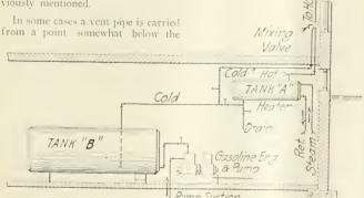
Fig. 2-Typical water supply arrangement
