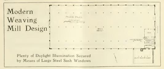
THIS mill presents a somewhat new departure in the design of weaving mills, especially as to the daylighting of the interior.
