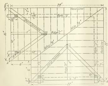
Fig. 2—Common Rafter Developed on the Plan-With the Top Pitch Projection, Width of Facia and Plancher Levels Known, the Heights of the Plate Cao Be Determined
