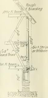
Fig. 3-How Temporary Interior Sheathing Board Braces Should be Nailed to Floor Beams as Each Tier is Placed
