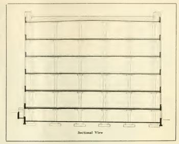
and rapidly nearing completion. It is expected that it will be ready for occupancy by February 1st, 1923. The floor plan shows the location of the different columns, in the length of the structure they are placed 24 feet on centers and in the width 22 feet on centers.
