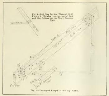
Measure in from facia line A, measuring on a level line, 2 inches, the width of the projection, locating wall line B. Measure down on facia line A, from the top edge of the rafter, 5/8 inch, the width of the facia, locating plancher level F.
