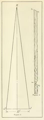
siding inclines one-half inch from the perpendicular. There are 120 half inches in half the diameter, so it will require 120x4½ equal to 540 inches, or 45 feet, to reach from J to K. Siding cut with a
