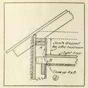
Fig. 4 shows the best detail for insulating the upper floor where the hoists are dropped below the eaves to afford room space in the attic. The open space A and B should be closed up with tight sheathing and a perfectly tight floor laid. Any good wall board can be used to cut off space A.
