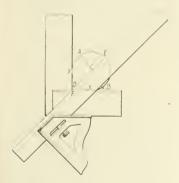
Place the two squares on the end of the pole or shaft to be centered, and draw a line across the face of the work Revolve the shaft, and draw another line. The result will be lines A, B, and D. E, crossing at C, which is the center of the circle.
