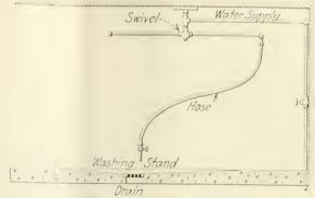
Fig. 1-Convenient hose arrangement for washing
