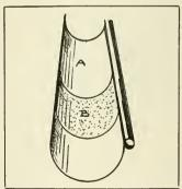
ing the edges of the lining to prevent the wind from getting between the lining and the metal eave trough. I repaired several troughs in this manner two years ago and they are in good condition at the present time. In the sketch A is the lining of roofing or canvas, B the mastic paint and C the eave trough to be repaired.—D. W. Daly.
