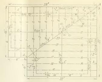
Fig. 1-Plan of Hip and Valley Roof of Unequal Pitch From Which Layout Is Made
