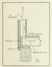
Fig. 1, showing air space between the studs and bow the air is carried by convection through from basement to attic, carrying the heat to the outside air. Also shows method used for stopping up space between studs with block at floor level, may be used in both old and new jobs.
