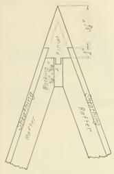
Fig. 2-Details of Finial-Section Through S-S, Figure 1
