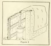
The studs and rafters are usually four feet on centers and braced by nailing stay lath to the inside of the framing.
