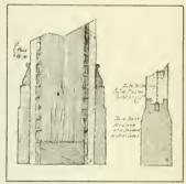
Section Through an Ordinary Lath and Plastered Partition Contrasted with a Corresponding Section of the Solid Plaster Partition and Base—Both Sections Are tha Same Size
