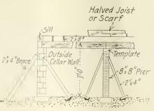
Fig. 2-How Foundations, Piers and Walls Ought to be Temporarily Braced While Green or Until the Mortar Has Set
