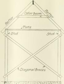
Fig. 5-Temporary Diagonal Inserted to Prevent Movement Before Sheathing and Inside Partitions Are Set
