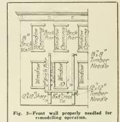
This brace should not slope at a greater angle than 60 degrees and be of good spruce or yellow pine timber, not necessarily new, but sound in heart and fibre, which may be ascertained by striking it with a heavy hatchet or maul. If it gives forth a clear ringing sound from the blow it is good, if not, set it aside and don't use it, as it may be decayed in the heart or dangerously split somewhere not visible.
