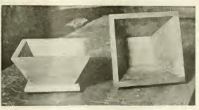
Fig. I-Assembled hoppers, the one on the left showing a miter joint and the one on the right a butt joint
