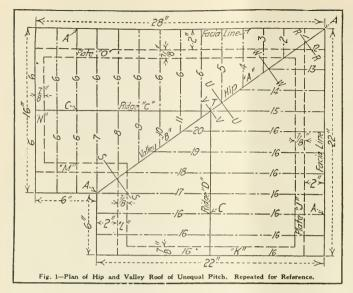
D to F is the developed length of the long common rafter.
