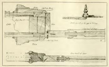
Plan of One-Half of an Ordinary Door and its Jamb in Contrast with the Corresponding Parts of the Doorway Devised by Mr. Flagg-Both Plans Are to the Same Scale
