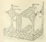
Fig. 8 Braced Angles or Corners, so as to Give Clear Passageway
