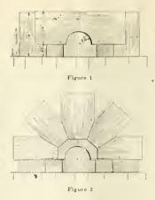
Figure 1 shows the first step toward working in this design. Two good 12" shingles are tacked on lightly, compasses set at 415" and the first circle struck. Take them off and saw perfectly to this struck line, put 'em back with nails in same holes and then nail thoroughly and this completes our figure one.
