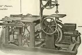
Furnished with Built-in Gasoline Engine, Self-Contained Electric Motor or for Belt Drive. Portable Variety Woodworker with 20-Inch Band Saw.
