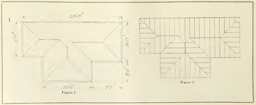
inches on centers their runs diminish 24 inches, hence lengths are shortened successively 2 feet, 478 miches for common and jacks, and 3 feet, 1½ inches for hips and valleys, thus, figure these lengths and work them on the diagram, which now completes a working plan for the whole reof.
