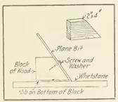
The base of the block is gonged out with a wood chisel leaving a slight elevation at each end which rest upon the surface of the whetstone when in use. The bit is slipped into place, and the screw tightened to hold the bit firmly and the edge brought to the proper shape by light, circular motions.
