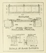
dows should be hinged to the outside of the roof and swing upwards. Suitable hooks should be provided so they may be adjusted from within. The cross section drawing illustrates the method of making the water tight joint between the roof and frames when closed.
