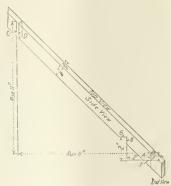
Fig. 3—Developed Length of Long Common Rafter No. 16
