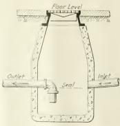
Fig. 4-Form of gasoline trap
