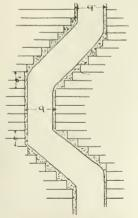
Section of Chimney Flue
