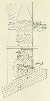
The arrangement of the bottom rail is the secret of its efficiency. Any water that might work up by capillary action would drop off at the quarter circle space. The other details are self-explanatory.—J. S. Adrianzen.
