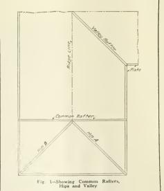
for the same rise and rim are the same length, and the center line along the top edge of each lies in the same plane as the top edges of the common rafters. This plane coincides with the under side of the roof-sheathing. With unbacked rafters this plane still passes through this center line on valley rafter, but not through that
