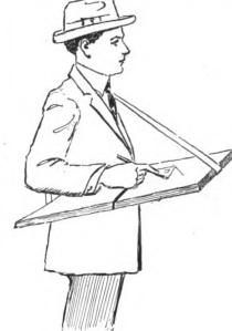
inches square each, with the hingesunderneath, when opened. The strapsare attached at opposite ends in the manner illustrated below. The strapis slung over the left shoulder, with the board under the right arm. When carrying, this is folded and the strapwrapped over, forming a compact unit that can be carried in the brief or letter case usually carried by the employee.—G. A. Luers.
