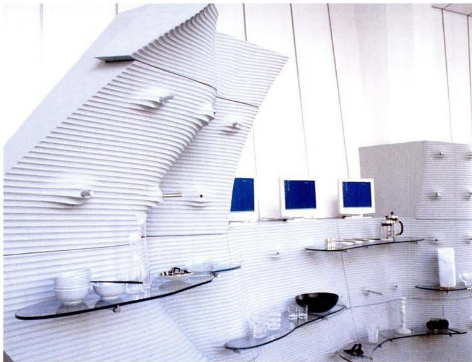
Machined lines delineate the contours of Lynn's forms. Far left: Renderings show the flowerlike Alessi Tea and Coffee Piazza 2000, made with a technology invented for stealth aircraft in which titanium "super-plastic" is heated to 900 degrees Fahrenheit. Above and left: In a Stockholm showroom interior, CNC-milled walls undulate with precision.
