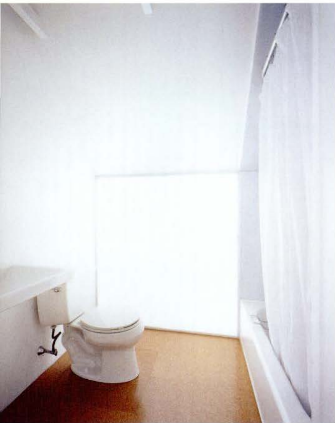
Upstairs, simple porcelain pieces such as a Kohler toilet adorn the modest master bathroom (above). Beneath the downward-pitched ceiling, a polycarbonate-panel wall brings in light from the south-facing skylight behind. i p. 154
