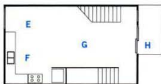
Second-Floor Plan E Dining Room F Kitchen G Living Room H Balcony
