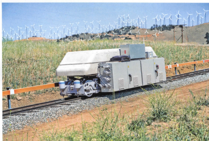
A weighted rail car on a 1,000-foot test track that ARES built in Tehachapi, California, near one of the country's first large-scale wind farms.
