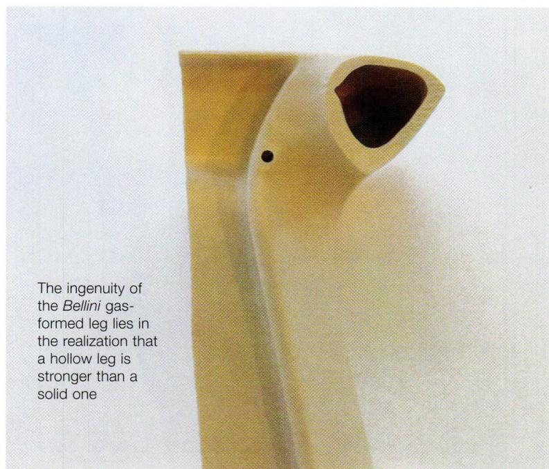
The ingenuity of the *Bellini* gas-formed leg lies in the realization that a hollow leg is stronger than a solid one
