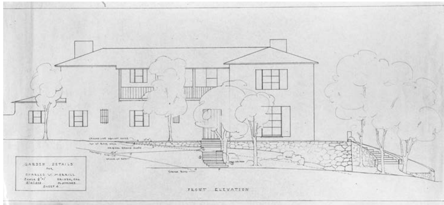
Above: This simple elevation drawing for the Merrill garden (Orinda, 1938) shows the entry stairs and walls at the front of the house. These features are among the few that are extant. A note shows the location of the road to the garage meaning the drawing precedes revisions to driveway approach and the path to the front door. Merrill Garden Details, Sheet 4. Drawings courtesy the owner of the property.
