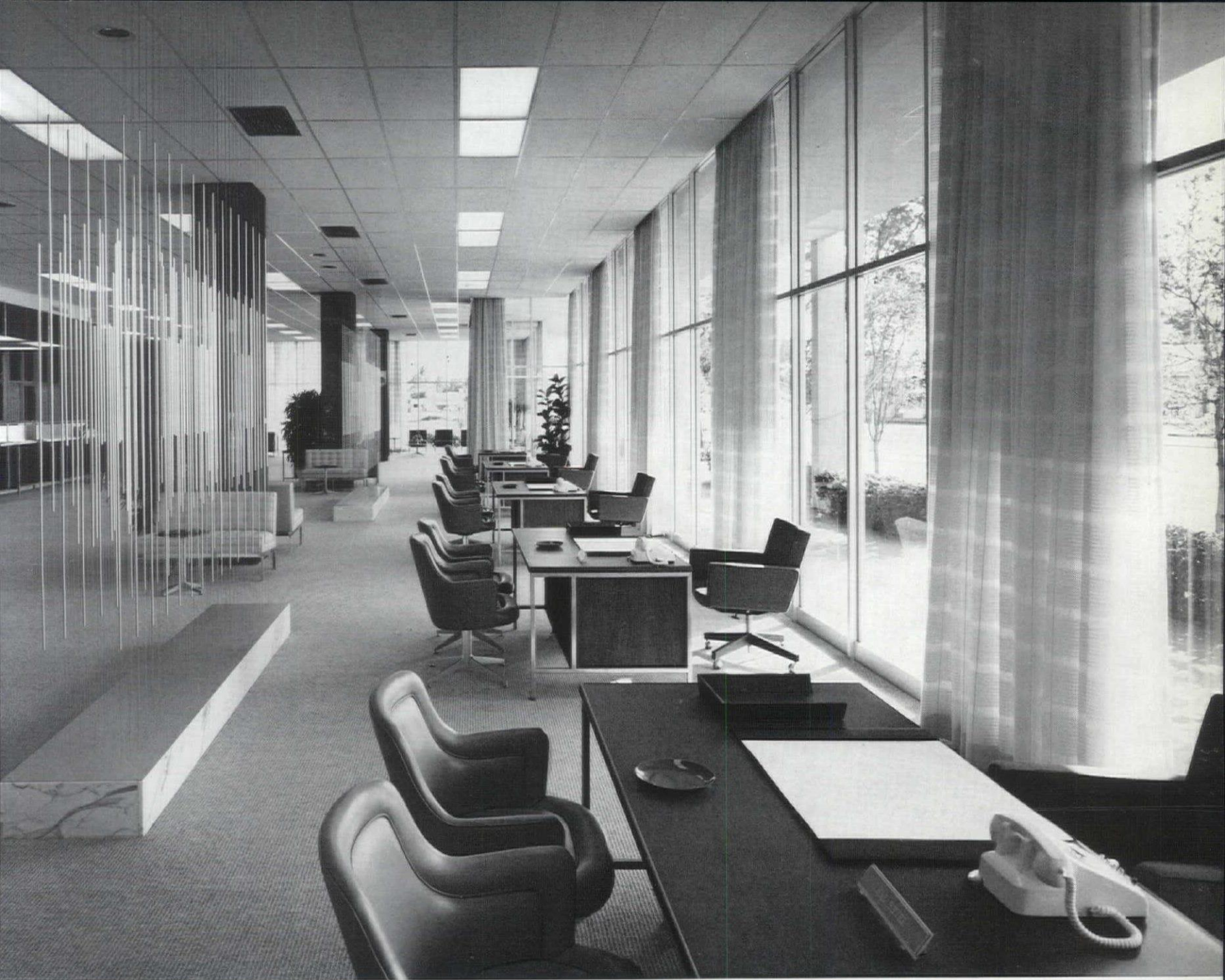
Officer's section of main banking area is partitioned by unusual dividers of cable and stainless steel rods, suspended to ceiling.
