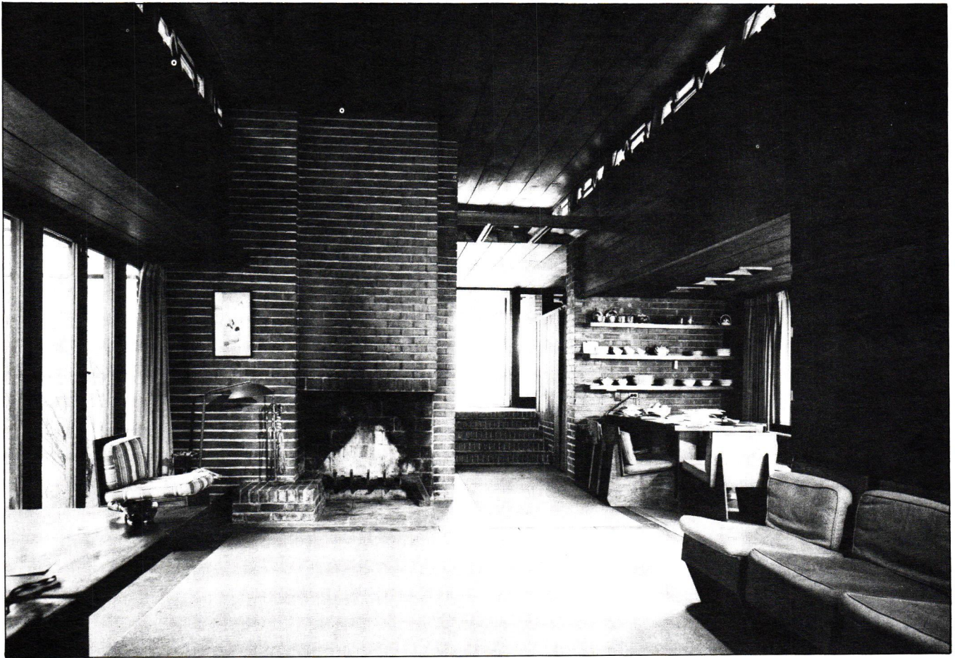
Fig. 13. Frank Lloyd Wright, Loren Pope House, Mt. Vernon, Virginia, 1939, interior. Two floor levels and three ceiling heights are visible in this photo. From the entrance (center, rear) several steps lead down, and the height of the ceiling is raised in scale with standing activities of the living area. For seating areas, around the dining table to the right and between the fireplace and the windows at the left, the ceiling is much lower (HABS/Boucher).
