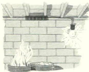
**FIRE FINDER.** An appliance so sensitive to sudden heat that it will instantly give warning of the smallest fire is now available. It is attached to the ceiling, or hidden from sight behind a grille in the ceiling and by its reaction to the presence of fire will attract attention to the hazard before it has had time to spread. When any sudden rise in room temperature approximates 20 degrees per minute the fire finder will sound an alarm.
