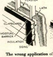
The wrong application of heavy building paper to the outer wall of a house over the siding is often responsible for the imprisonment of moisture within the wall section. Plaster defects may result from this
