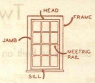
The critical points in a window are illustrated above. A well-designed window will remain secure and completely weather-tight throughout its life
