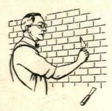
Solid brick walls seldom leak unless the mortar joint has loosened. Loose joints should be cut out and repointed with a heavy mortar mix. A coat of colorless waterproofing will bond up and waterproof the average wall. Any hair cracks may be disregarded.
