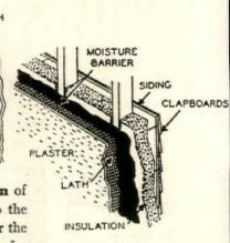
The proper application of a moisture-proof barried to the warm inner side of the wall inhibits the flow of air-borne vapor to the insulation and consequently prevents the occurrence of condensation in the wall
