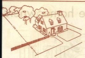
Open sweeps of 150 ft. or more are counteracted by setting the snow-guard 20 ft. from the weather side of road. This allows for down-drift
