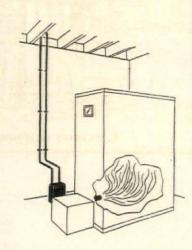
Wasteful consumption of oil is eliminated if burner nozzles are properly adjusted to produce a clean and hot flame. The ignition system should be adjusted to insure quick starts and cutoffs to prevent any dripping of the unfired fuel
