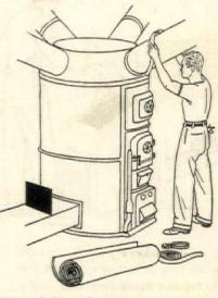
The sliding damper which controls the flow of fresh air to a warm air furnace may be kept closed in Winter; the air used may be recirculated. Covering the warm air ducts with insulation insures delivery of more heat to all the rooms
