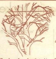
Boughs or branches that whip against service wires should be trimmed to prevent breaks
