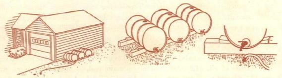
Hidden behind the garage of this home are three 50 gallon drums holding an emergency supply of fuel oil. Emptying them into the tank is simple Drums are mounted on timbers and wedged in place. Garden faucets are tapped into each and oil is run through a section of hose to the main tank
