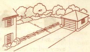
Short sweeps, under 50 ft., do not work up a great amount of down-drift. In this case the snow-guards may be placed within 6 ft. of edge they protect
