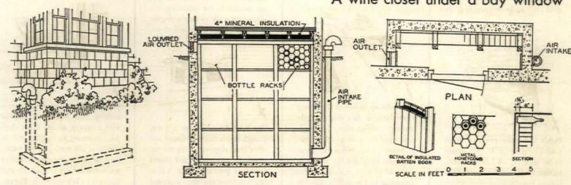
Ventilation in the proper amount is furnished by the circulation provided by the intake pipe and louvre. Racks are spaced and divided as shown
