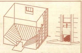
Dust-proof coal bins with sloped metal bottoms are simple to construct. The usual window gives access to bin, and guillotine door controls supply
