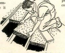
Most modern insulation is available with a moisture barrier fabricated as an integral part of the insulation. When this is not the case, moisture-proof paper can be laid or nailed on the room side of the insulation as shown
