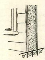
Increasingly cold is the temperature inside your walls, working from the inside towards the outdoors. If moist, warm air seeps into inner wall, it will reach a point where colder temperatures will condense it
