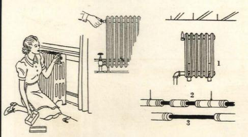
Radiator valves on steam systems mean much to their operation. Cheap or defective valves are an extravagance. Petcocks on hot water radiators should be opened to draw off air which accumulates at the top Exposed heating mains will give as much heat as a wall radiator (1). Short exposures (2) of the pipe do not chill the system as long exposures (3). Obviously, the wall radiator is the safest and best solution
