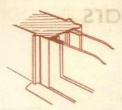
Storm sask should be used on all windows regardless of their location. The air space between the sash provides Winter insulation
