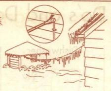
Sleet storms may load exposed wires to the breaking point, unless they are properly hung from a cable or put underground
