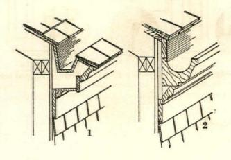
Wood gutters are ornamental as well as practical. Most popular types are the built-in gutter (1), which is not evident from ground level and is flashed on both sides as well as on the bottom, and the solid-type gutter (2) resembling a heavy moulding and only partly flashed. The use of wood to greatest extent is essential to national defense
