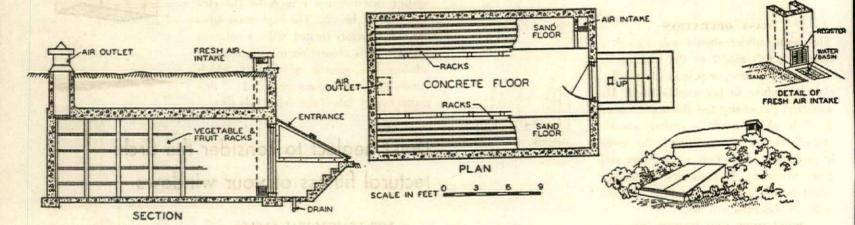
Ample storage is provided for fruit and vegetables in still another design. A steel door assembly and steps give access to the entrance The racks are constructed in open pattern which prevents molding of their contents. Ample vents provide necessary circulation of dry air
