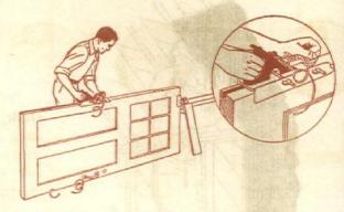
Rabbeting or grooving the edges of the door is done with a rabbeting-plane. This can be set to provide a groove of the proper shape and width. (See detail.)
