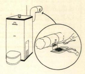
Soot accumulates rapidly where the damper controls the smoke pipe. Most dampers are equipped with a clean-out door at the bottom. This should be opened several times during the heating season and the damper chamber cleaned out
