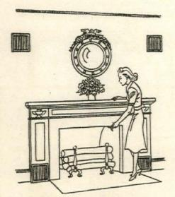
Dampers in fireplaces should be kept tightly closed unless the fireplace is in operation. Cold and draughty floors can often be traced to the lack of a damper. Fireplaces equipped with a heat circulating feature become very effective heaters
