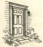
Solid doors which make the entrance hall dark can be corrected by installing a stock assembly having side lights as shown. When the old door frame is removed the wall is cut away on each side to the extent of one stud. The trimmers are doubled up and the new assembly erected in place. This improvement involves less work than might be expected by the home owner. At right are details for the builder
