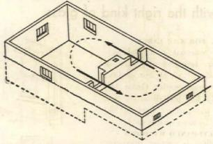
Unexcavated cellars or partly excavated cellars should have small windows to provide for free circulation of air. If these areas are isolated and kept tightly closed they are liable to create damp and unhealthy conditions. Even where the partitioning wall is of solid construction these openings can be made without too great a building expense Sound advice solves common problems in home construction inside the house and out
