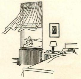
Fully opened windows are unnecessary and extravagant. If the window must be opened wide the heat should be turned off so as not to chill the system or to keep the boiler in constant and very wasteful operation throughout the night
