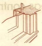
Double-hung windows especially need good weather-stripping in order to be perfectly weather-tight yet work smoothly
