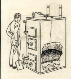
Deep beds of fire are economical rather than wasteful. The fire bed should be deep enough to reach from the grates to the bottom of the fire door. Shallow beds of fire burn out rapidly and are extravagant of fuel. Keep the ash-pit clean
