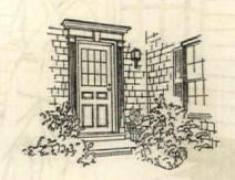
Doorways adjacent to a corner might be improved by a latticed enclosure which extends to the wall. For Winter weather solid battens and storm door are buttoned in place. The design shown provides for an additional closet for the storage of skis, sleds and Winter equipment which are best left outside the house. The canopy shown is of copper or sheet lead but could be simulated in plywood construction
