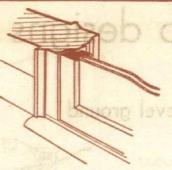
Double-glazing, a new development, takes the place of storm sash. Two sheets of glass are here fixed in a single sash
