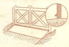
A bead or molding at the bottom of garage doors prevents an accumulation of ice beneath them
