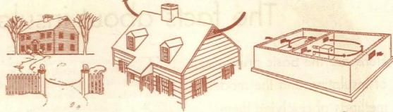
Closed for the winter, this home, even though insulated, might suffer damage from condensation Ventilating louvers in the attictend to prevent accumulation of moist air from within the house
