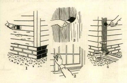
All materials benefit by paint. Clapboard (1) should be scraped before painting. Mill-work and trim (2) should be thoroughly sanded. Unpainted wood-work (3) can be preserved and beautified with oil. Light-weight metal, such as down-spouts (4), should be kept painted
