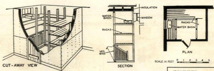
A practical substitute for the underground storage room can be constructed in a corner of the cellar. Water pans provide the required humidity Insulation in both the walls and ceiling of this corner store room is required. A window is essential for providing required ventilation How? See the more than a hundred practical decorating ideas in our October Double Number
