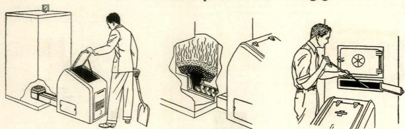
Automatic coal stokers may be installed in practically any type of heating system. A very compact unit requires filling only once a day. They burn an economical grade of coal, are practically dustless and are very quiet and efficient A worm-gear or conveyor shaft carries the coal from the hopper to the retort. Fresh coal is forced up, as required, through the bed of fire which insures complete combustion of the gases. There is practically little or no ash left over
