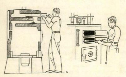
Clean flues inside the boiler are essential for the economical operation of the heating plant. As little as three-sixteenths of an inch of fly ash or soot covering the flues cuts the performance of the boiler in half. Clean-outs give access to the flue surfaces. Our pictures show, above left, ash scraped forward in upper flue and, right, pushed back to drop into ash-pit into which a shovel can be inserted for cleaning. Cleaning should be done twice during the year
