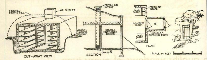
Root cellars provide the best storage for fruit and vegetables. The earth which is excavated is used to cover the structure and insulate it Double doors and small vestibule help to maintain an even condition within. Ventilation is essential and provided by intake and outlet Sand floors are used beneath the shelves and furnish the required amount of moisture. A concrete slab provides good footing in center
