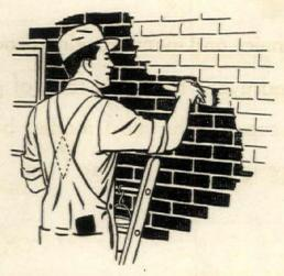
Brick walls benefit almost as much as wood does from a good painting. Small cracks and minor defects in the mortar joints will be filled and made weather-tight by it
