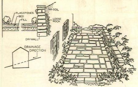
Drainage on a hillside frequently presents a problem in rolling country. A practical solution for a house whose walls face a hill is found in the low retaining wall and flagged terrace. This provides a barrier between the wall and the natural hill drainage, insures a dry cellar and a dry wall. The terrace in such a location provides privacy as well as utility, and is extremely attractive
