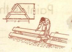
Snow-horses make very efficient snowguards. 6 ft. lengths are readily handled. Construction, 2 x 4 ft. legs and 3/8 in. boards
