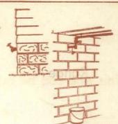
Outside hose connections should be shut off and drained off at outlet in the cellar
