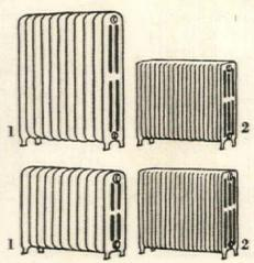
Modern design of radiators permits a 30% reduction in their size. Old-fashioned (1) radiators may be replaced with modern ones (2) that are almost half their size but deliver an equal amount of heat radiation
