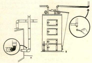
Insulation is needed at the fittings as well as on the long run of the heating pipes. Asbestos cement can be molded neatly around the elbows or tees, and does not require any bands
