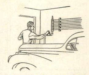
Heated garages need not be kept at same temperature as the house. Considerable fuel may be saved if the supply of heat is adjusted in a sensible manner. As garage heaters are generally at the end of a heating line they should be properly installed and controlled
