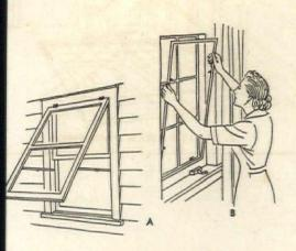
Storm sash and weather-stripping are the first steps in conserving your heat. The outside sash hung at the top, or the more modern doubleglaze which snaps into place inside the window, are equally effective if properly fitted and hung
