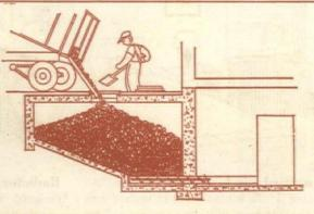
Coal storage can be clean and out of sight if a proper vault is built. A good suggestion is embodied in this concrete structure with an overhead manhole
