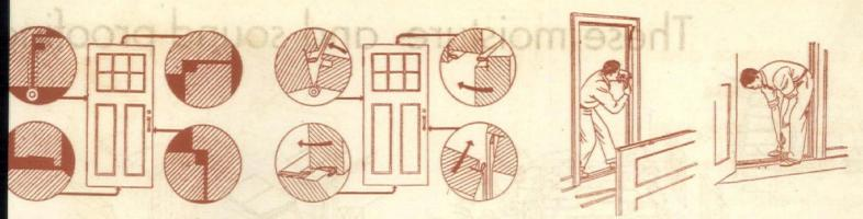
Each edge of door is rabbeted in a different manner, as shown above, to receive the weather-stripping of various shape and design.
