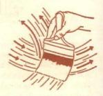
Thorough brushing in criss-cross pattern is proper for all flat surfaces
