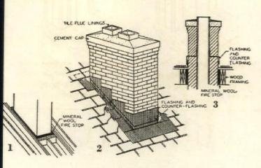
Good service may be expected from chimneys that are properly constructed. Flashing and counter-flashing (1) insure tight joint at the roof-line. A cement cap (2) provides proper topping. Fireproof material between the walls (3) of the chimney and the roof construction insure safety. This type of chimney work protects the interior of the house
