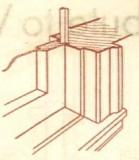
Weather-stripping should be of good quality and make positive contact with moving parts as shown in the casement above
