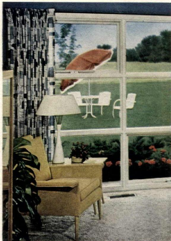
**GLASS INSULATES YEAR 'ROUND.** Seal out cold, heat and dirt with PPG's remarkable TWINDOW® insulating glass. TWINDOW is two panes of Pittsburgh Glass with a layer of dry air sealed in between. In summer, TWINDOW helps keep heat *out*; in winter, it helps keep expensive heat *in*. What a perfect way to eliminate storm windows!
