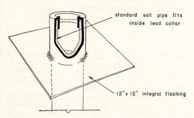
Levitt takes advantage of the shorter vent pipe projection sanctioned under the new national plumbing code to slip a flashing collar over the whole vent, thereby getting a more permanently waterproof job with almost no site labor cost at all. To save critical copper, the collar is made of lead.
