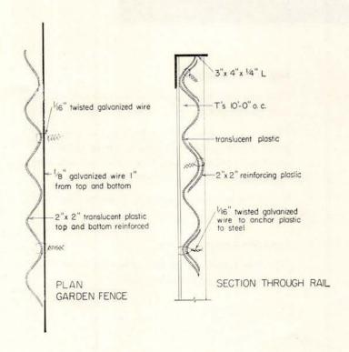
Because plastic material does not have to be drilled, detailing is simple.
