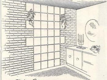
Dining Room 12" glass blocks worked in with the inside of a face brick wall interior
