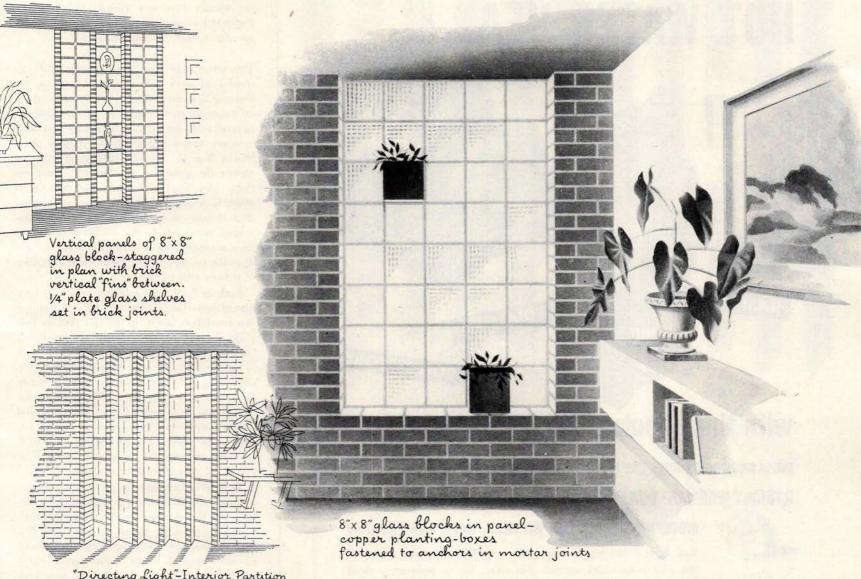
"Directing Light"-Interior Partition 12" x 12" glass block set at an angle with single brick "fin" separators between each row.
