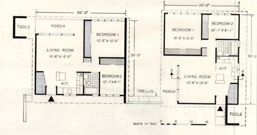
THE BUDGETEER has much in common with the two other new Levitt houses: Exterior wall panels are the same asbestos cement; slab, wall construction and interior painting are the same. But this is the Levitts' first flat roof. Kitchen has stainless steel sink, automatic washer, electric range, refrigerator. Bathroom is equipped like Levittowner. Each unit has 36 sq. ft. of outside storage.
