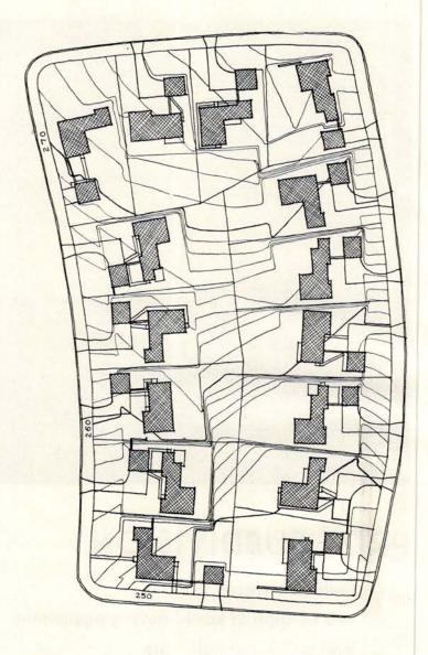
Typical block plan with 1' contours shows how level lots were terraced into the hillside. Note how contour lines gang up along lot lines, indicating the location of steep terraces and retaining walls.
