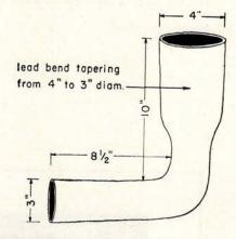
In earlier Levitt houses a lead bend below each toilet was made of 4" pipe. Now the lower portion is of 3" pipe, which saves about 4 lbs. of lead per fitting. The famous Jalonack plumbing tree will be used again. For photo see Feb. issue '51.
