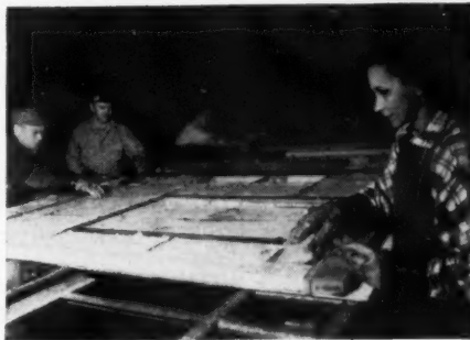
ELECTRONIC PRESSES set phenolic glue under pressure and heat generated by 60 kw current. Principal designer of the house, Electrical Engineer George W. Stanley, is at controls.
