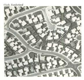
DO use curves, loops, cul-de-sacs to slow traffic, create visual variety. Use long blocks (up to 2,000') to reduce intersections, save on paving, utilities.
