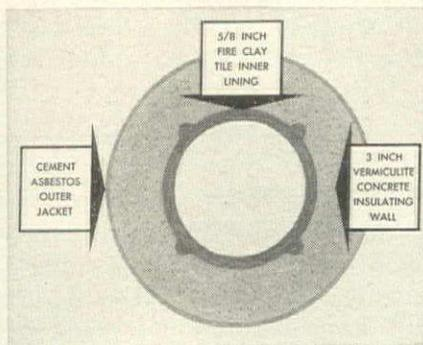
**Safe, permanent** masonry materials go into Van-Packer Chimneys. Flue sections have insulating value of 24" solid brick. 5/8" fire clay tile liner withstands 2100° F. Built to last.
