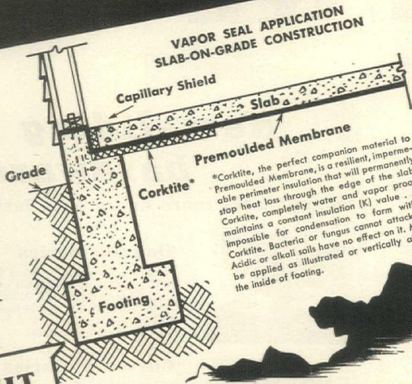
\*Corktite, the perfect companion material to Premoulded Membrane, is a resilient, impermeable perimeter insulation that will permanently stop heat loss through the edge of the slab. Corktite, completely water and vapor proof, maintains a constant insulation (K) value . . . impossible for condensation to form within Corktite. Bacteria or fungus cannot attack it. Acidic or alkali soils have no effect on it. May be applied as illustrated or vertically along the inside of footing.
