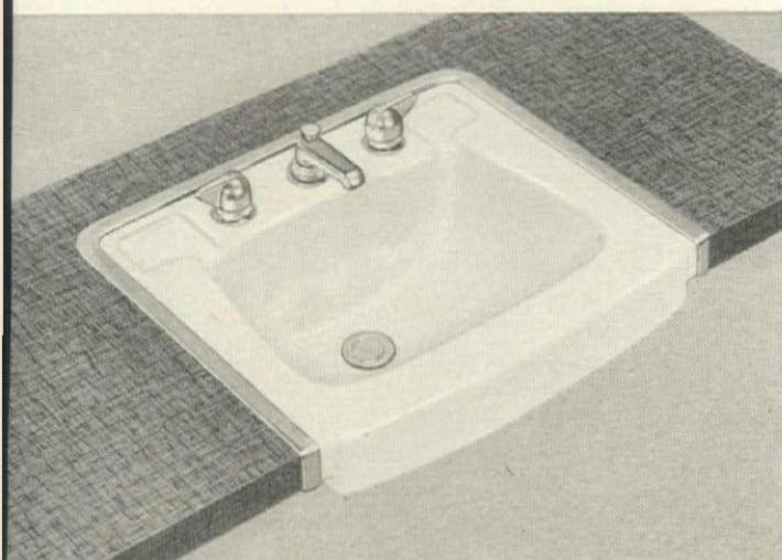
**Countess.** Newest low-cost counter-top lavatory, the vitreous-china Countess combines small overall size with big-basin convenience. Basin is wider at front (15½") than at back (14"). Overall size is only 20" x 17", and lavatory can be installed (if desired) in a counter measuring only 16" front to back. Bright chromium plated fittings, Dial-ese controls, indirect-lift waste. Basin has integral soap depressions.
