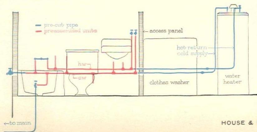
**Complete plumbing tree** is installed in 6" thick wall and shipped by Precision Built Homes. All kitchen and bath fixtures, can be included at builder's option. Cost to builder for this complete prefabricated plumbing package, including fixtures, for a one-bath \$10 000 house is about \$400. Builder saves up to \$200 a house, compared with cost of buying his plumbing locally.
