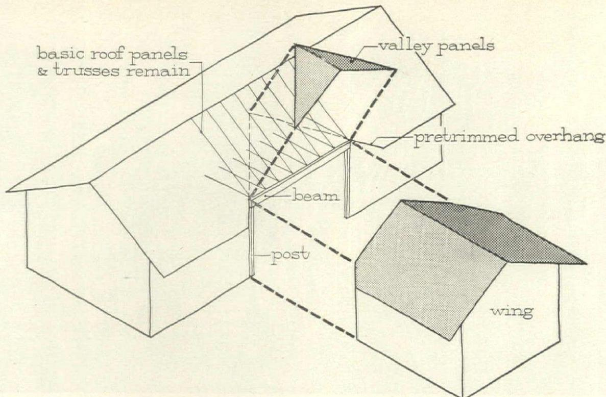
**Exploded diagram** shows how the breakout principle works. In this example a 24' wide wing is added to a rectangular house. Key to system is "dropped beam", usually 4" x 12", which bridges open space in exterior wall of main house where wing is to be added. Beam lines-up flush with top of adjacent wall panels, rests on two posts and provides support for trusses which normally rest on panels. Two precut triangular "valley panels" connect roof of wing with roof of main house.
