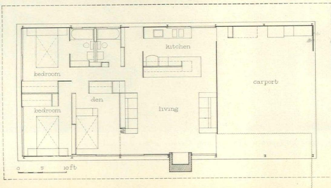
**3-bedroom, 2-bath plan** is extremely compact, saves space through elimination of fixed interior partitions. All were replaced by storage walls of veneered plywood.
