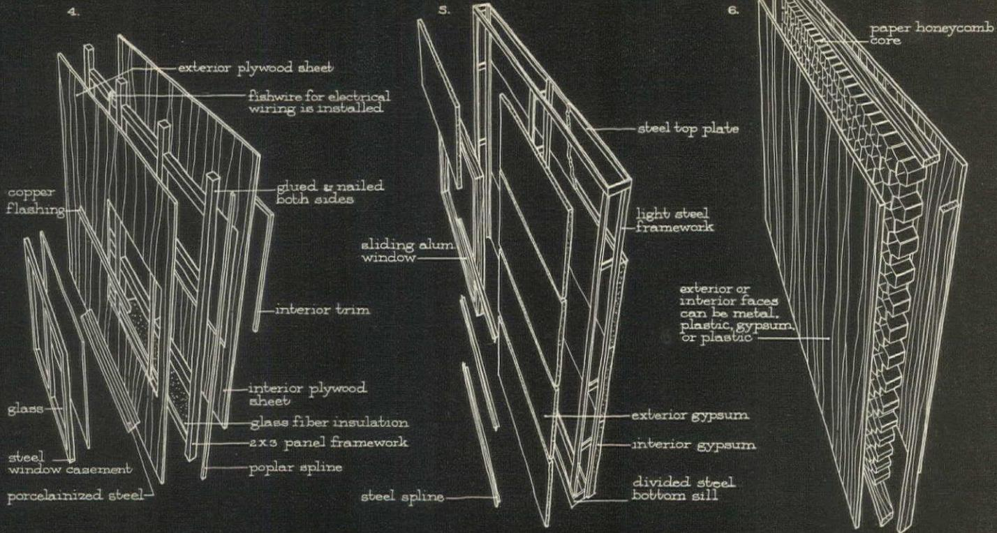
**Interior face** of this panel (US Steel Homes), unlike others, is factory-finished. A stress-skin panel, it utilizes a 2x3 framework to which plywood is glued and nailed. Panel is insulated, windows installed and glazed and provision is made for pulling through electrical wiring. Random scoring of interior face obliterates actual panel joint.
