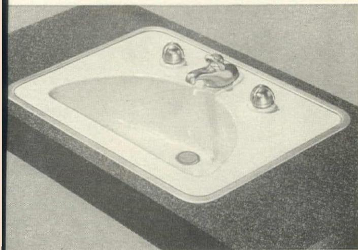
**Elayne.** Simplicity of design is the keynote for the Elayne's large semi-oval vitreous china basin—the largest basin of all Crane counter-top lavatories. Made of finest vitreous china in white or any of seven pastel shades, with Temple chromium plated trim, Dial-ese controls, lever action Securo waste for quick draining. Overall size: 27" x 20". Basin, 21" x 11".
