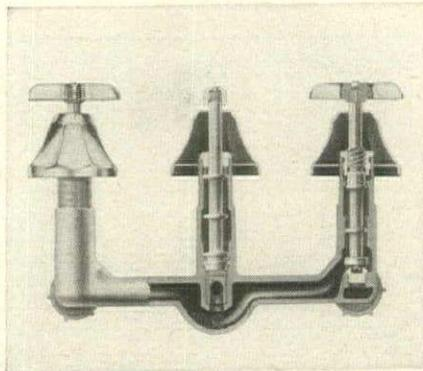
**n. SHOWER DIVERTER** changes water flow without altering temperature
