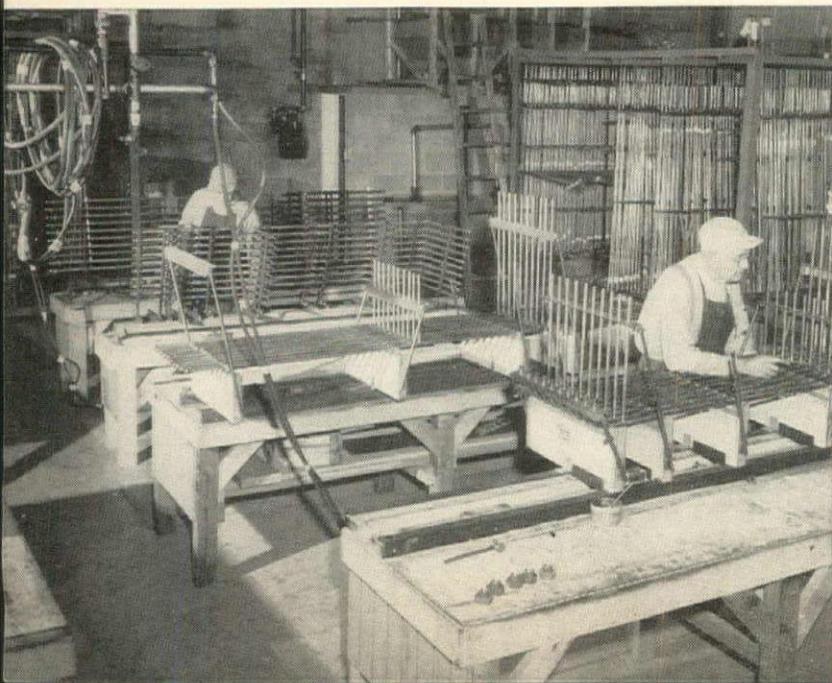
**Hot and cold water** supply manifolds are only partially assembled before shipment by National Homes. Final assembly is made at the house so builders can easily vary the hook-up to meet local codes and the different needs of National's line of houses. Cast iron drain pipes are also provided. Pipe manifolds in plan (below) are shown stacked in factory.
