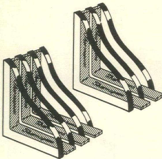
3 and 4-pane units are available for refrigerated cases and for unusually severe conditions requiring low coefficient of heat transfer.
