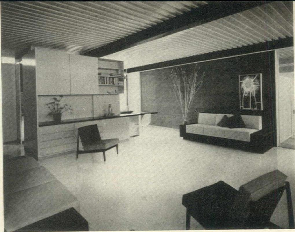
**Because** there are no interior structural supports, plan can be adjusted almost at will
