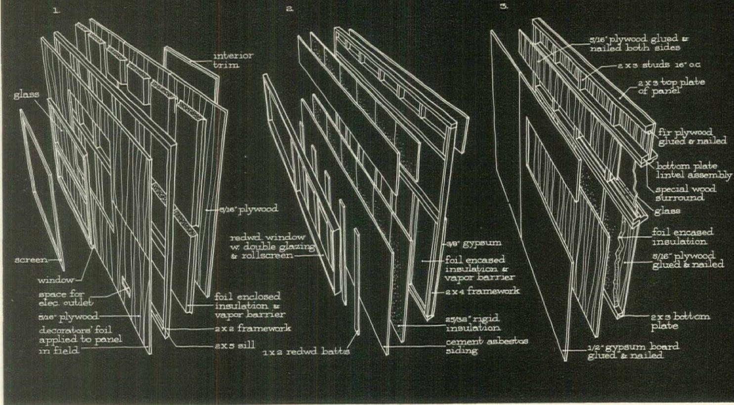
**Plywood**, stress-skin panel (New Century) is strong, thin, lightweight structure utilizing 2x2s for skeletal framework. Panels are joined by nails tongue and groove fashion and panel joints are hidden when decorator's felt is glued to interior, covered with texture paints. Windows are installed and glazed.
