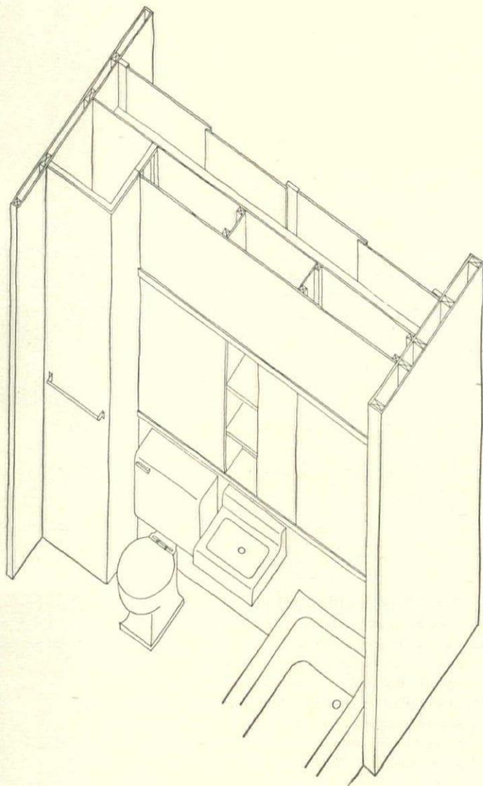
**Complete units** contain plumbing, wiring, domestic hot-water heater, chimney flue (furnace goes in crawl-space below floor). Shown left is two-bath unit of the type used in Kansas City suburb where the National Plumbing Code is acceptable. Details, above.
