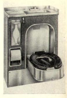
L. PACKAGED BATHROOM fits into one-third the space required for usual plumbing. Called Travel-Lav, it comes in two sizes. The smaller unit takes 85%" x 20" of floor space, has an overall height of 34½" and includes a foldaway toilet and stationary wash basin. The larger unit (not illustrated) is 31" x 39", 78" high, includes enclosed shower cabinet, medicine cabinet, exhaust fan and lighting as well as foldaway toilet and wash basin. Angelo Colonna, Inc., Philadelphia 34, Pa.
