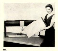
PREWIRED VENTILATING HOOD has a solid top designed with easy breakouts to accommodate three Trade-Wind ventilators. Prewiring cuts installation time, allows for a simple electrical connection after hood is fastened to the cabinet. Three-speed control, operated by a finger-tip touch bar. controls both ventilator and light. New hood is available in stainless steel and satin copper or in antique copper. Trade-Wind Motorfans, Inc., Rivera, Calif.
