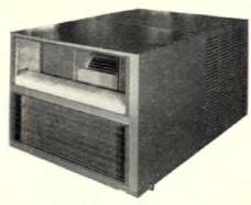
kk. YORK SUMMER CONDITIONER, called Pathfinder, is designed for attic installation independent of the heater, but can be connected to warm-air heating ductwork. Since unit is air-cooled, no plumbing is needed but unit must be located near a gable for access to outside air. The 2- and 3-ton sizes have dual compressors giving two-stage con-
