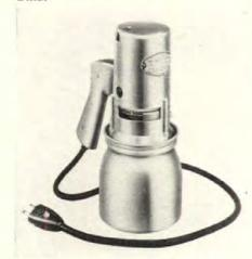
**WW NEW PAINT GUN** is designed like a centrifugal pump. Rogers Rotary Magic Painter is powered by a self-contained Westinghouse motor that spins the rotor blades at speeds up to 22,000 rpm, pumping the paint from a twist-on aluminum can. Dial on handle regulates
