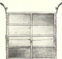
FLEETWOOD '57 (left) is Crawford Door Co.'s big new line of garage doors -72 single-door styles and sizes are available, and there are 60 double-door combinations. Doors come two to eight panels wide and from four to five sections high. All models need 3" side room, 111/2" headroom. Company also offers a special double horizontal track which cuts required headroom to 21/2". Crawford Door Co., Detroit, Mich.
