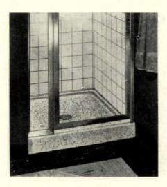
FLOOR with integral threshold can be ordered as a 32", 36" or 40" square, 36 x 40" corner or 48 x 38" rectangle. "Monterey" floor comes in four colors, a wrought brass drain body is cast with the floor as is a galvanized-bonderized steel flange. NAHB show-goers will also see company's line of packaged shower cabinets in a variety of price ranges for many kinds of home installations. Fiat Metal Mfg. Co.
