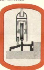
... Moisture cup in track halts condensation from flowing onto floor or carpeting.
