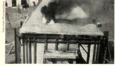
Flame test of new fire-resistant chemical was made in this structure built of fire-retardant wood. Structure was fired with gasoline and outside air was blown in to speed combustion (fans at bottom). Above, the fire breaks through roof, after 45 minutes of gasoline feeding.
