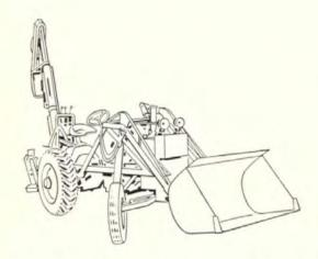
Back-hoe and high-lift combination Schmitt calls single most valuable machine, cost \$4,500. "Any builder of 10 houses a year needs one as much as he needs a power saw." See also No. 7; 17.
