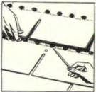
Sun heat activates the adhesive and creates a secure bond which keeps the shingles lying flat even in winds up to hurricane force. But, the spaces between the individual seals allow for drainage and therefore prevent rapid deterioration.
