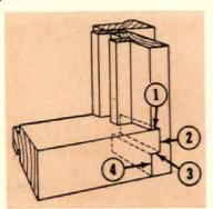
RIGID SILL has four bearing points to prevent warping and assure watertight protection.
