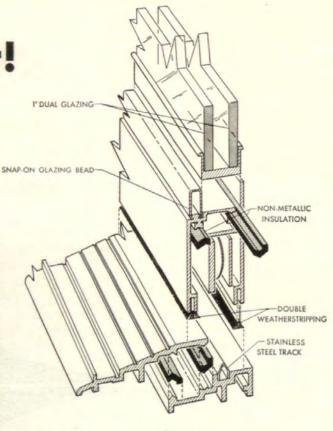
Secret of Ador Insulated Thermo Door is shown by this exploded view of threshold and sliding unit bottom rail. Black areas are non-metallic strips of insulation. They effectively seal interior metal surfaces from the outside. This restricts heat flow, overcomes condensation. Note also double weatherstripping, inside and out.
