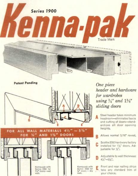
Kenna-pak, prefabricated adjustable wardrobe header assembly, is complete with steel header, Scottie Series 2050 sliding door hardware and wood nailing strips for wardrobes using 34" and 136" sliding doors. Completely packaged, Kenna-pak cuts labor and installation costs while adding to the beauty of sliding door wardrobe installations.
