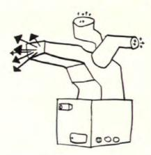
speed and adjusting registers for proper air temperatures in all rooms. It should be done on a cloudy day or at night when there is no sun heat to contend with. If the system is not balanced some rooms will get too much heat, others too little.
