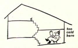
ceiling duct! Result: floors remain cold, and air temperatures vary as much as 32° from floor to ceiling!
