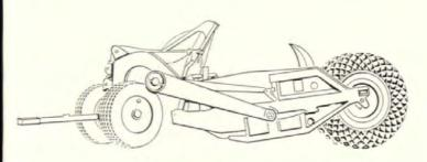
Big scraper is used to grade lots, cut through streets, cost \$10,000. Big machine is too heavy to be hauled by small bulldozer so Schmitt bought big second bulldozer. See also No. 13; 20.
