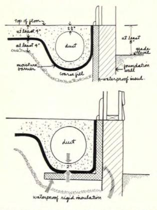
Slab houses also need heat supplied at floor level—preferably through a perimeter system which will surround the slab with a "fence" of warm air. Further advantage: feeder ducts spreading out under the slab provide an extra bonus of radiant heat.
