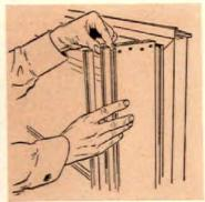
JAMB LINERS are easy to remove . . . adapt frame to walls from 4½" to 5¼" on Malt-a-Matic, Malt-a-Glide and picture units.
