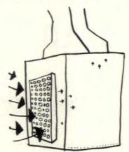
can be pulled through them. Before a house is sold, the filter should be cleaned or replaced.
