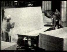
IN THE FINISHING DEPT., check carefully for grade and appearance. Check accuracy of dimensions and thickness. Apply grade-trademarks.
