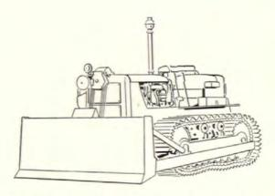
Big bulldozer, used to push earth and haul big scraper, is needed at 50-houses-a-year level, says Schmitt, cost \$20,000. "I just completed \$20,000 worth of grading with one." See No. 13; 20.
