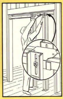
2. Install uprights After header is up, it's a simple matter to secure split jamb and split stud to header brackets.
