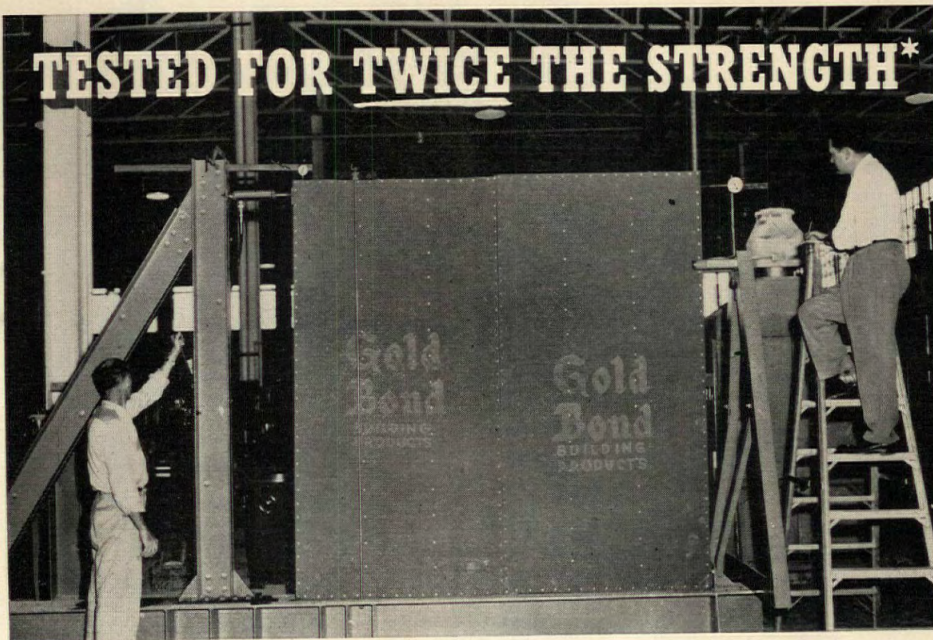
Gold Bond Insulation Sheathing takes the "racking pressure test". Test and results authenticated by Pittsburgh Testing Laboratories.
