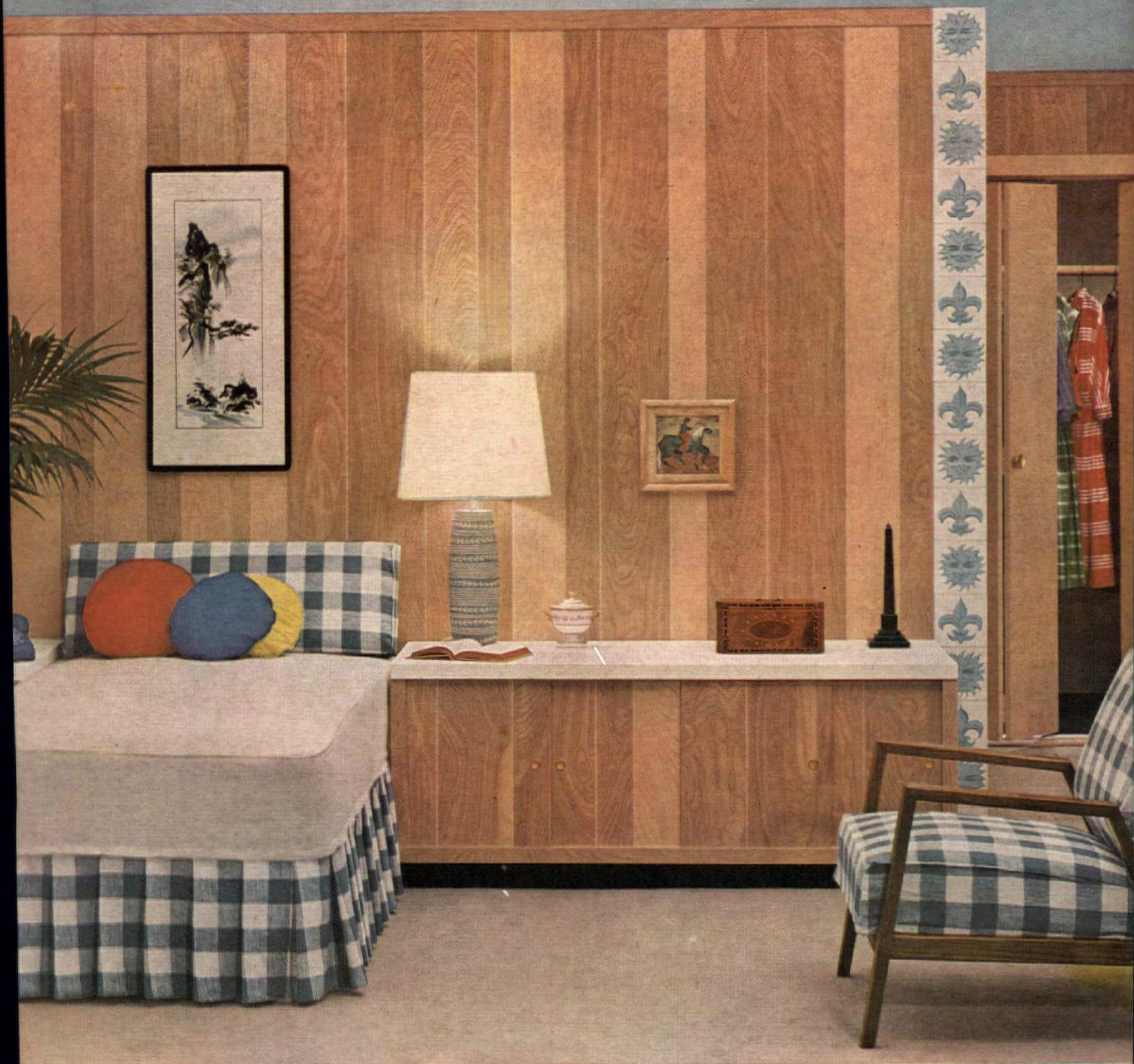
Wall is of 4' x 8' Birch V-Plank* panels, with matching Weldwood hardwood moldings. Weldwood Bi-Fold closet doors (right) are birch-faced, have cores of non-warping Novoply.®
