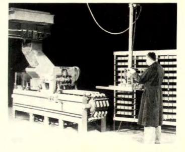
**d.** Cavitex masonry block, seen in wall construction above, is produced by a new stepped-up continuous process machine, see right, which receives a precision-measured mix, then tamps, trowels and forms it into the Cavitex blocks.
