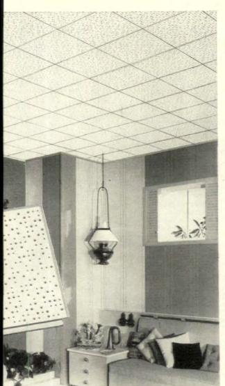
Each Fibretex Panel contains hundreds of small noise traps which absorb up to 75% of the room noise that strikes them. Panels are prefinished in white. Furnished with Lightning Joint or with square edge. Panels are 12" x 12", and 12" x 24", 1/2" and 3/4" thick. All panels come in uniform and random drilled pattern.
