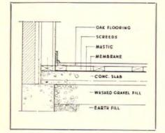
1 Start with a well-constructed concrete slab. Use a surface moisture barrier of 15-lb. asphalt felt or polyethylene film embedded in mastic.
