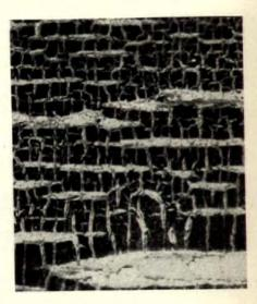
ALLIGATORING is the final stage of checking, resulting from improper mixture of pigments on too much oil in the prime coat. Cracks reach down to bare wood.
