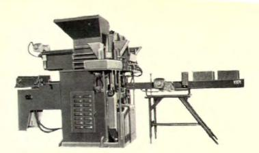
c. Pacer block masonry, left, can be turned out by the machine above at the rate of 5,000 per day.
