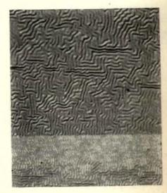
WRINKLING comes from coating paint too heavily if paint is not made for thick coat, or from the wrong combination of vehicle and pigment in the finish coat./END
