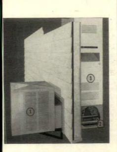
v. This central air conditioner slides through the outside wall of the houseand right into the furnace, see above. It does away with the need for long refrigerant tube connections because the cooling coils (2) are a part of the condensing unit package that goes through the wall into the furnace plenum (3). Refrigerant tube connections are made by manufacturer. Condensing unit (1) remains outside house.
