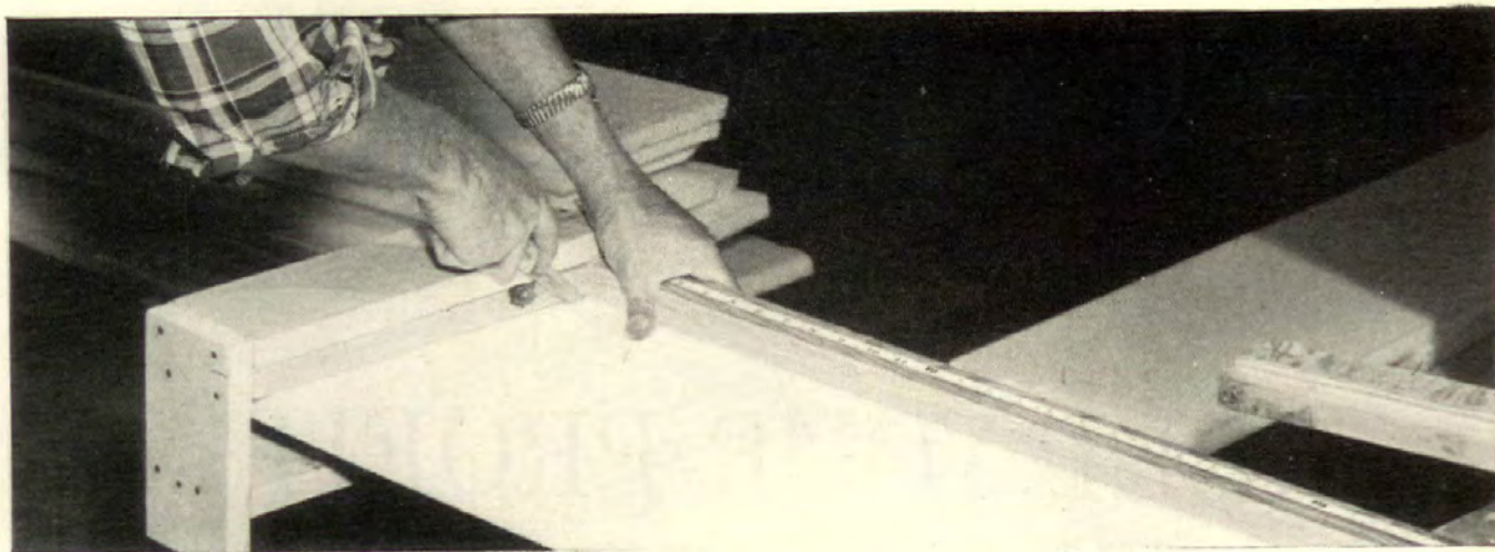
"CUTTING AND SHAPING Styrofoam® is almost effortless," says Mr. Walrod. "It can be scored with a knife and snapped off in any desired size."
