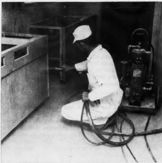
HOT-SPRAY EQUIPMENT , which uses water jackets or heating coils to make heavy bodied paints less viscous, can match the coverage of the usual three-coat finish in one pass of the gun.
