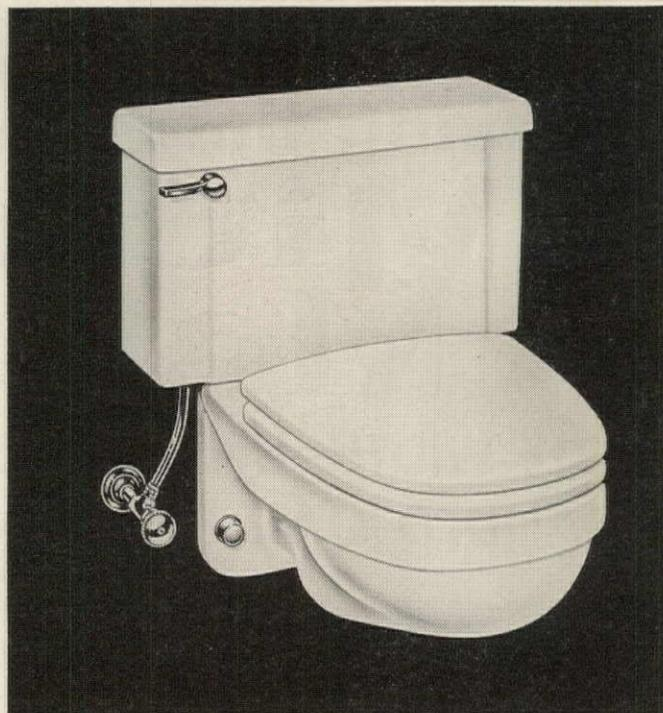
Since the unit has horizontal discharge, drainage collection can be above the floor, in the wall behind the unit. And since the floor underneath is clear (at its lowest point, the unit is 1 1/2" off the floor), cleaning is easy and flooring can be installed without fitting around toilet base. Tank is standard size: 12" h., 21" w., 7" deep. Bowl is 15" h., projects 26". American-Standard Plumbing & Heating Div. New York City.
