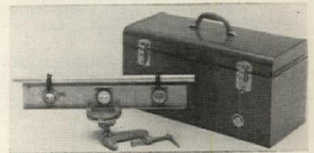
**n. Magelite sighting level** comes complete with sighting tube (that has both a buckhorn opening tube that has a peep crosshair sight) mounted on the 18" protractor level. Turnplate head is calibrated and adjustable and the 4" graduated circle is movable so angles may be read from zero. It operates in 360° with graduations of 2½°. \$29.95. You can get tripod of heavy gauge tubular aluminum as an accessory—it is interchangeable with C-clamp mounting. J. H. Scharf Mfg. Co., Omaha.
