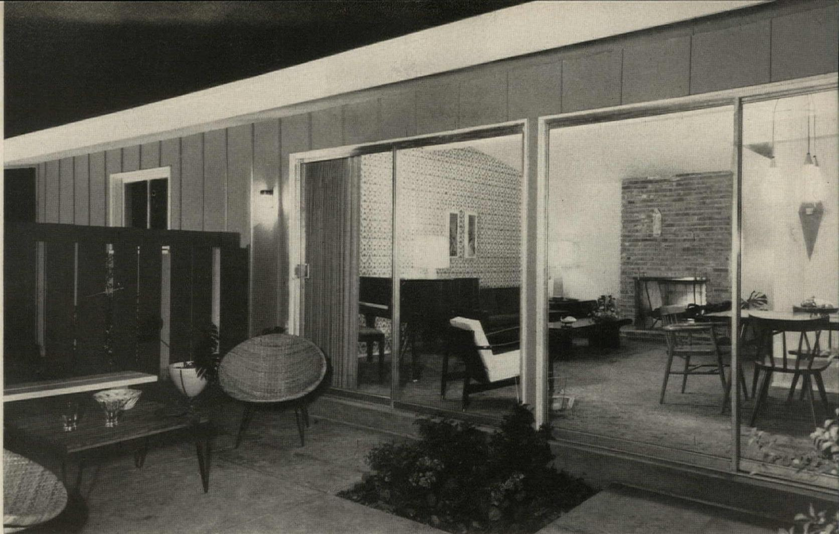
**LIVING-DINING AREA** (a) opens onto large terrace through 8' sliding glass doors. Sidewall is 5/16" asbestos board with battens 16" o.c.
