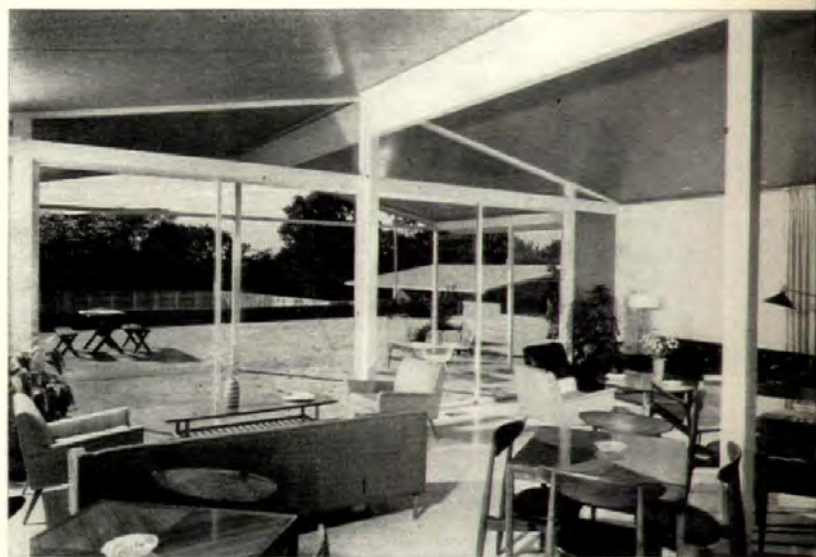
INSIDE THE HOUSE , no painting is needed because the interior finish is anodized permanently into the panel's aluminum skin.
