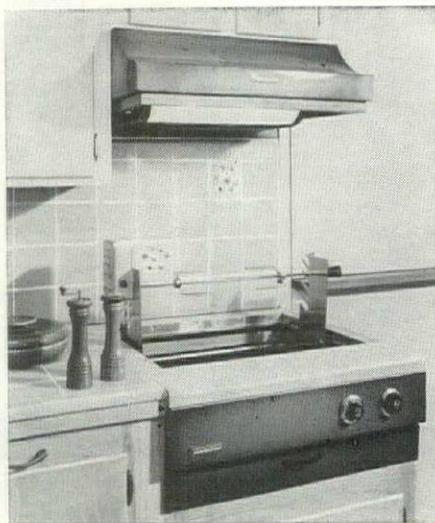
**"Electramic" broiler** contains two special heating elements above a bed of ceramic coals. The ceramic is removable and can be washed. You can install this charcoal-less barbecue in kitchen, family room or on a patio. The broiler mounts on any cabinet 24" square and 28" high. That will place the hardwood cutting board top (which fits over the unit) about 1¼" above a 36" counter top. Installation should be made to include a ventilating hood, company says.
