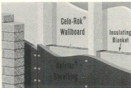
OUTSIDE AND INSIDE, the Mark 58 features superior wall construction: Celotex Insulating Sheathing for added insulation and greater strength; Celo-Rok® Gypsum Wallboard for smart, durable interiors.
