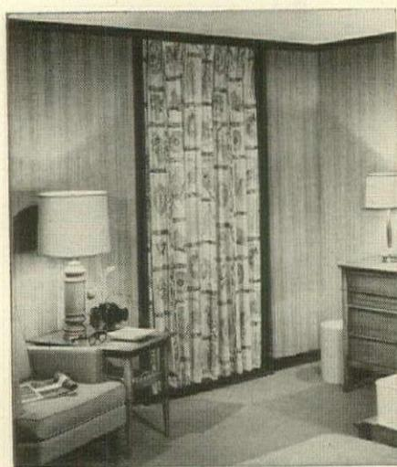
**Predecorated sheetrock** from US Gypsum, is available in three new finishes — Cherrywood, Sablewood, and Ranch Pine. The 3/8" gypsum wallboard is predecorated with a face paper, suitable for use in remodeling as well as new construction. The surface of the board is washable, and can be waxed or varnished for extra durability. Sheetrock comes in 4' widths.
