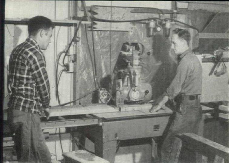
**2** Lumber is cut on radial saw with two labor-saving attachments: 1) metal tape on reel (left of saw) is hooked onto end of lumber, saves time in measuring; 2) pneumatic cylinder moves saw across work, leaves operator's hands free.
