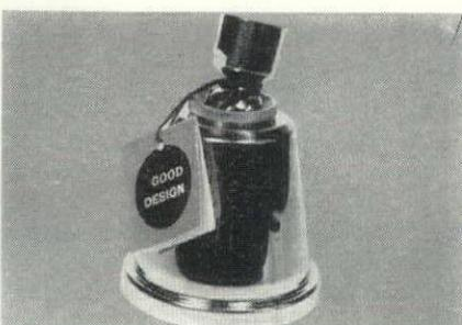
**Shower head** gives 60 streams of water which can be tuned to tingling, gentle or foamy washing action. Live rubber diaphragm in shower head is pierced with 60 slits. Water enters main body of shower head which is a large mixing chamber for incoming water to reach uniform temperature. Metal plate gives it a further swirling action.
