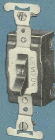
▲ **MECHANICAL QUIET SWITCH** Fully enclosed. Operates in any position. Will withstand the high inductive loads of fluorescent systems and take the full rated capacity of tungsten filament lamp loads. Rated 15A.-120-277V. AC only. This new 277 volt rating permits this switch to be utilized in modern 4-wire electrical systems now being installed.
