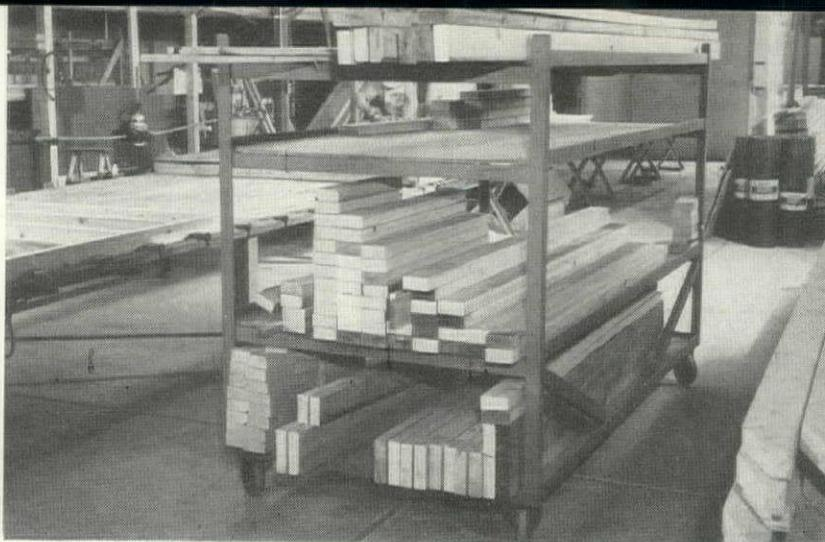
**3** Cut-to-size lumber is stacked on this four-shelf hand truck, which is pushed to assembly jig by handler. Truck was designed by shop superintendent—holds enough material for a half-day's work. Frame is welded steel; shelves 3/4" plywood.
