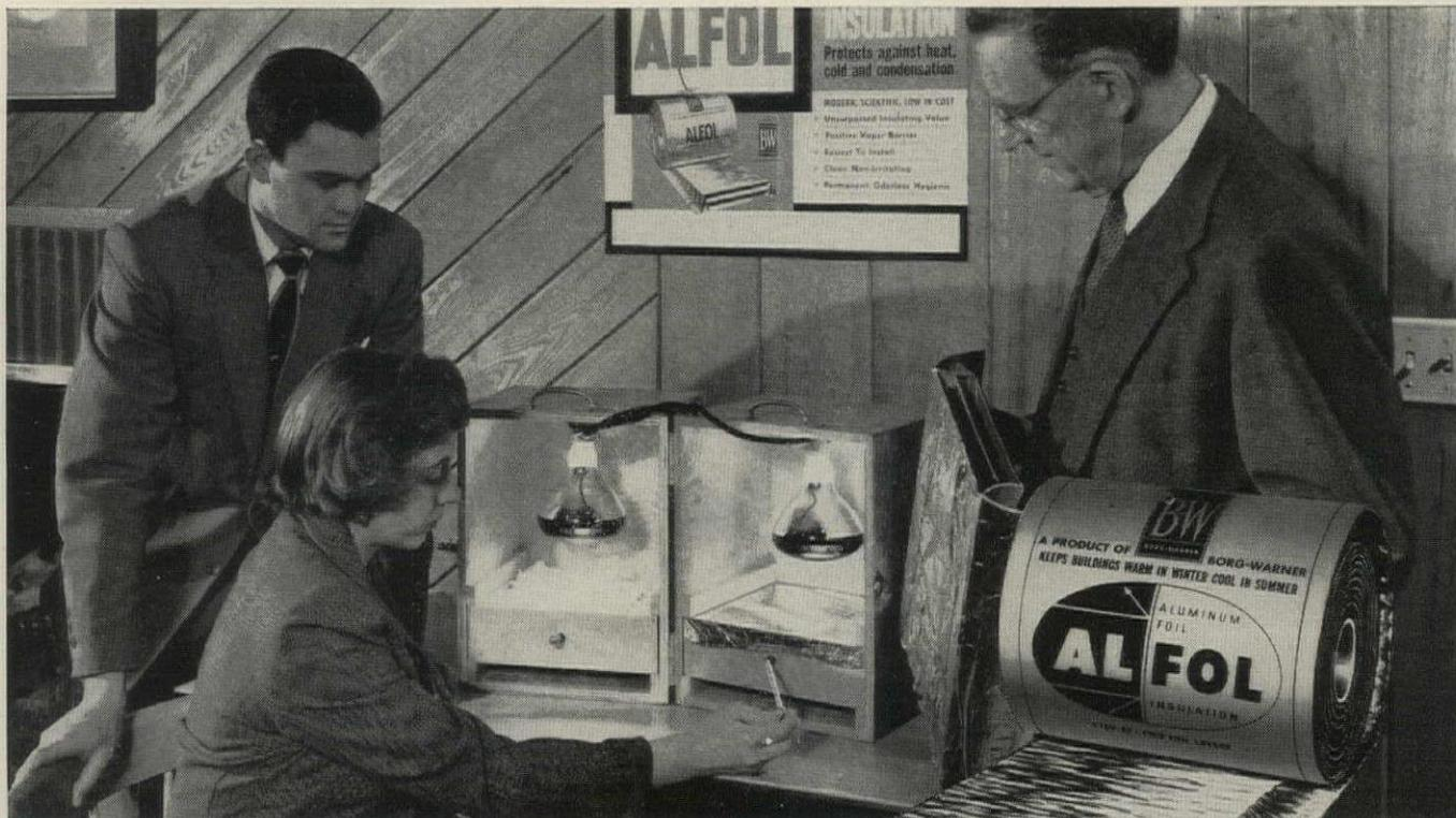
After just minutes of heat lamp exposure, temperature under the aluminum foil panel (right) measures some 12° cooler than temperature under bulk insulation. Conditions are identical.
