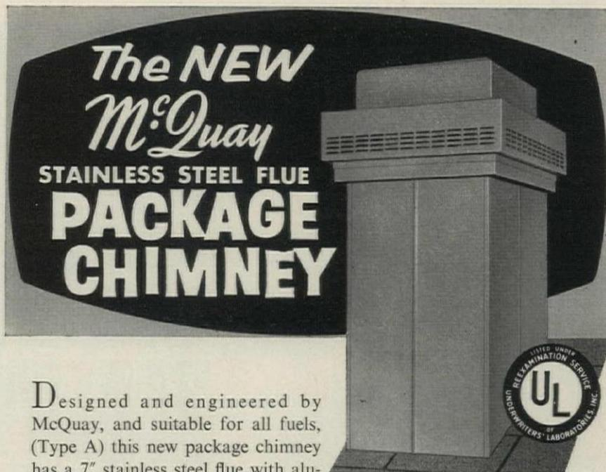
Designed and engineered by McQuay, and suitable for all fuels, (Type A) this new package chimney has a 7" stainless steel flue with aluminumized steel interliner and outer casing. The interliner is supported by the exclusive McQuay stainless steel tension spring spacers for strength, rigidity and durability.
