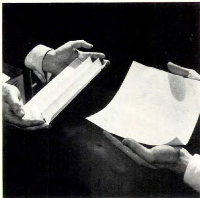
FOLDED PAPER demonstrates the strength of "folded plate," shows how same section might sag when diaphragm strength is not used correctly.
