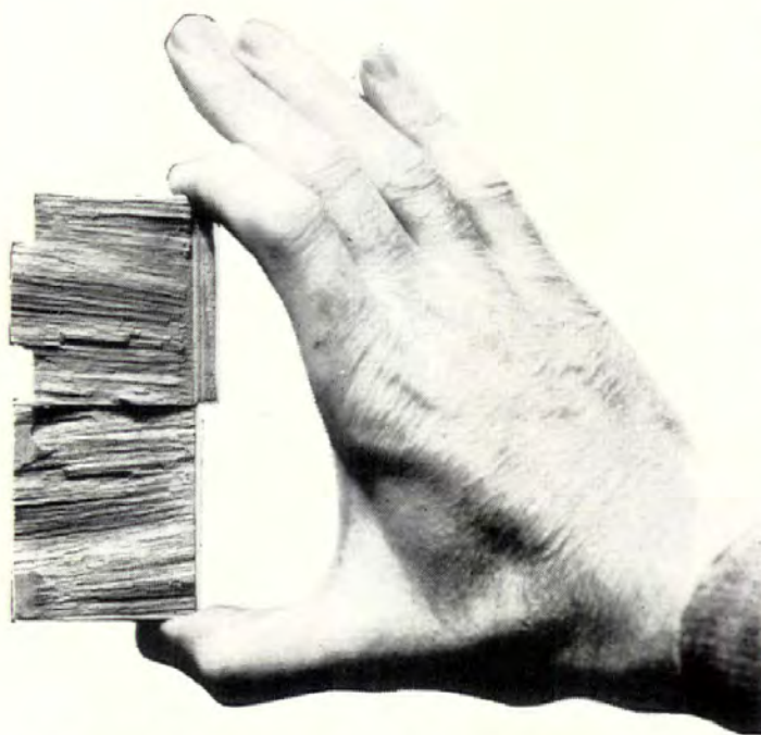
GLUE SHEAR TEST shows how test blocks break through the wood fibers, not the glue line—proving glue bond is stronger than wood.
