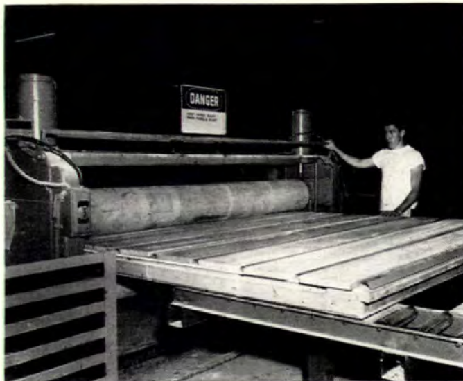
Rollers press aluminum sheet to wall panel, as boards protect ridges.
