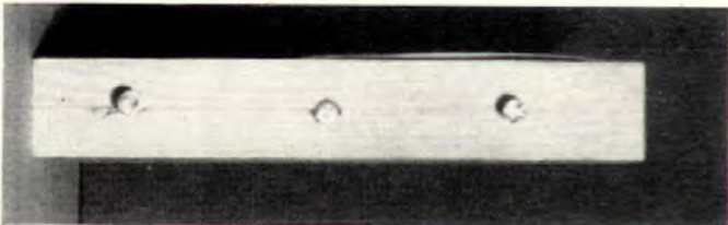
LAMINATED 2x4 made of two 1x4s has glue bond strong enough to withstand three spikes driven right through glue line.
