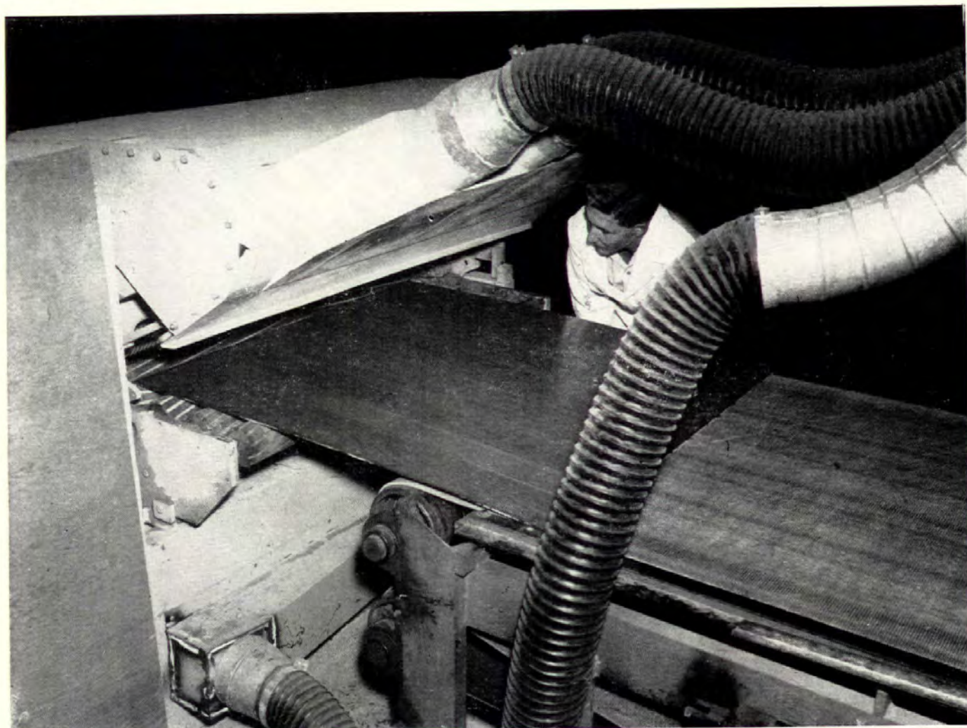
PREFINISHING is a fast (97 minutes) and highly automated process on production lines like this one at US Plywood's Orangeburg, SC plant.
