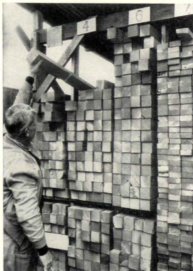
NUMBERED BINS are used to stockpile specially cut and notched pieces. Numbers guide the teamster (required by the union), who selects and loads lumber and is unfamiliar with dimensions. Says one building supervisor: "We like to do everything by the numbers."
