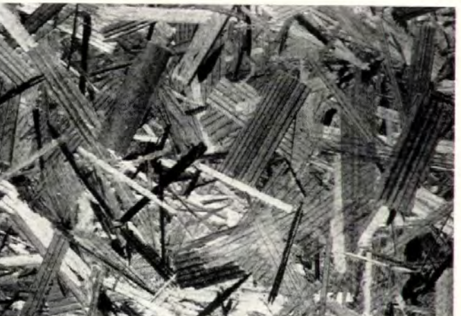
PARTICLE BOARDS are strong contenders in the decorative paneling field. Wood flakes and wafers are colorful, and have distinctive grain.
