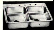
New low-priced sink in stainless stee is offered in the new Ekco Standard line, listed at retail prices 16% lower than the deluxe line introduced last year. The sink is made of 20-gauge 18-8 stainless in an over-all satin finish. The new line has the same white acoustical undercoating and comes in the same sizes, shapes, and depths as the deluxe line.
