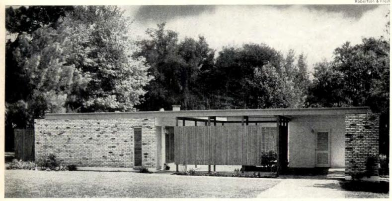
FACADE is lengthened by brick panels extending beyond end walls and by strong roof line tying together house, patio fence, and carport at right.
