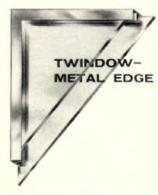
TWINDOW—METAL EDGE. This type is ideal for large windows and where maximum insulation is needed. It's made up of two panes of 1/4" clear-vision Plate Glass, with a 1/5" sealed air space between. Its stainless steel frame, a TWINDOW feature, eliminates bare edges . . . makes handling safe, quick and easy.
