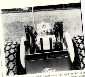
Power steering on new Ford tractor turns full right or left in le than one turn, absorbs kickback when driving over rough ground
