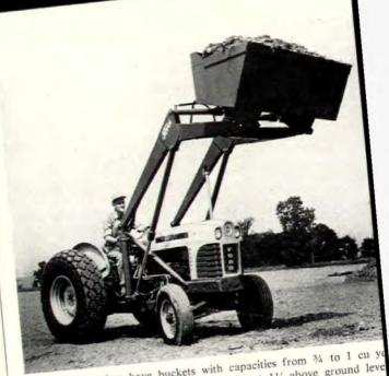
Ford-made loaders have buckets with capacities from 3/4 to 1 cu y will break out 5,500 lb, lift 2,500 lb almost 11' above ground leve
