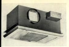
New ventilator light from Fasco is aimed at the builder market. Unit is prewired, easy to install in 6" rafter space. Rough-in box fits 16" oc joists, inner box blugs into the rough-in box quickly, and grille snaps on. Duct 4" in diameter connects unit to roof jack. The light is supplied by two 60-w bulbs mounted behind milk glass diffusers. The fan is made of glass rods and is designed so air flows freely.
