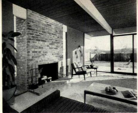
LIVING ROOM (a) has big fireplace mass flanked by fixed glass panels that break wall, help open room. Ceiling is 2" redwood t&g topped by ½" Fiberglas insulation and built-up roof.
