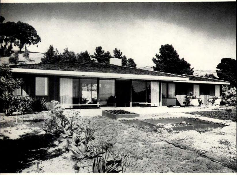
OUTSIDE LIVING ROOM you see how 27' wall of sliding glass opens room to terrace. Wall faces south, but 6' overhang keeps glare off glass.
