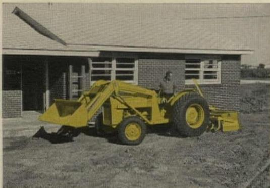
The Work Bull 202 with the Backhoe detached (you take it off or put it on in five minutes) and the M-F Scarifier-Scraper hooked up will scarify, level, back-fill, or scarify and level at the same time.
