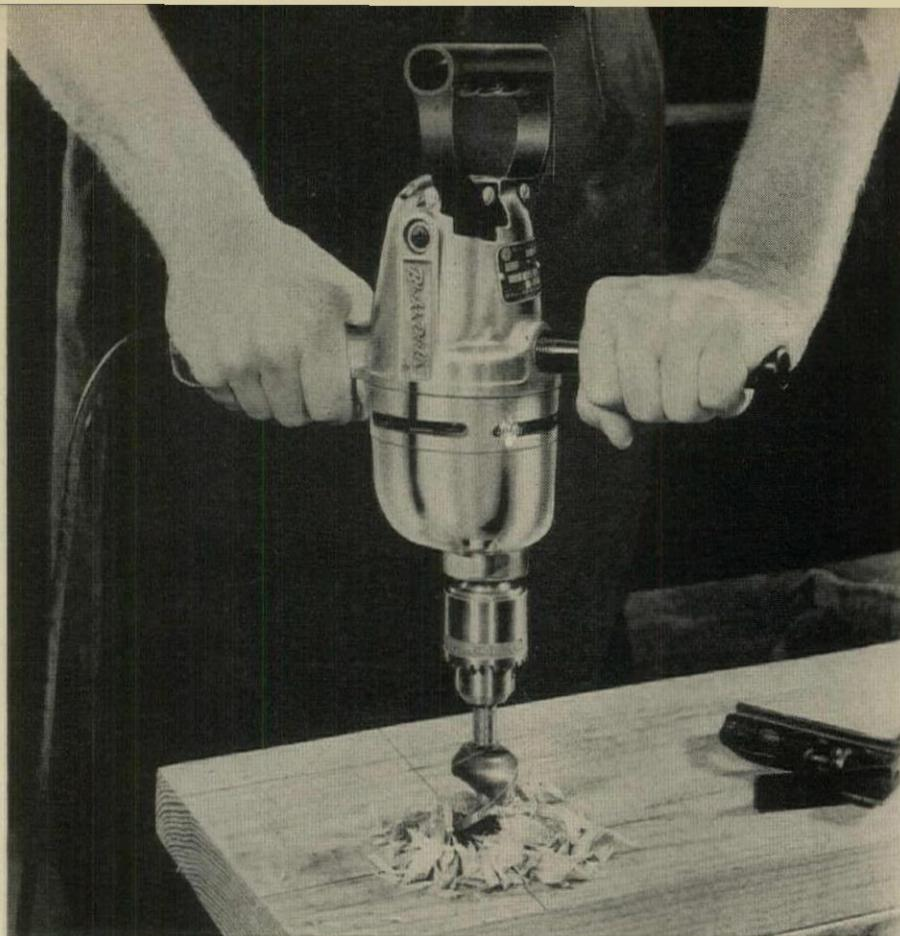
**BLACK & DECKER'S U-21-A** will drill 1/2" holes in steel, 3/4" in masonry, 1" in wood, or hole-saw 2". Geared chuck takes 1/2" shank.
