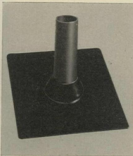
**Neoprene vent flashing** can be installed by one man in five minutes or less, the makers claim. Collar is double-seal, is made for standard vent diameters and 3-in-12, 4-in-12, 5-in-12, and 6-in-12 pitches.
