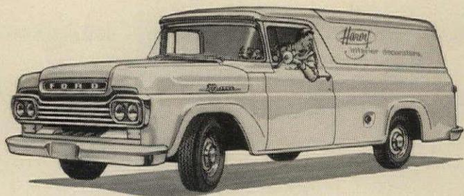
**Ford's F-100 panel** offers 158 cu. ft. of load-space—husky all-steel body and weather-sealed plywood floor.
