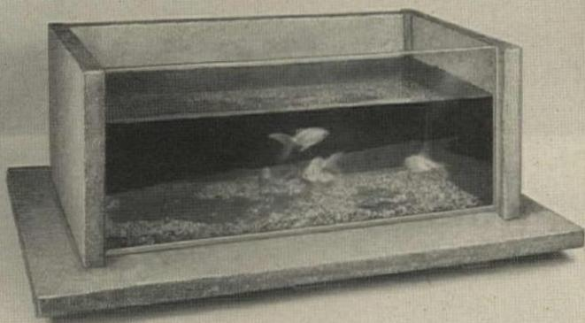
We built a Bildrite goldfish bowl to prove the point that Insulite sheathings are really water-resistant. And yet, it's a remarkable fact that moisture vapor *passes through* these asphalt-impregnated boards—helping to maintain dry walls and excellent insulation.
