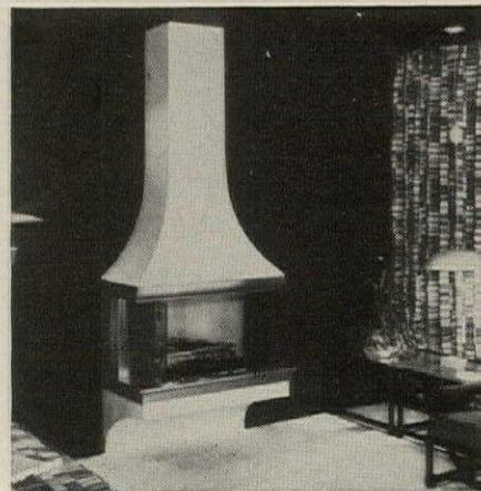
**Uni-bilt wall-hung fireplace** is factory-made, complete with chimney. Ceramic firebox is held on a cantilevered hearth in an enameled housing. Baffles and insulation insure safe exterior temperatures. Chimney is stainless-steel lined with galvanized outer casing, aluminized middle flue. Exterior housing and rain cap are also galvanized. Prices, fob distributor, \$380-\$511, depending on roof height. Tile hearth, \$31, and grate, \$9, are extra. Vega Industries, Syracuse.
