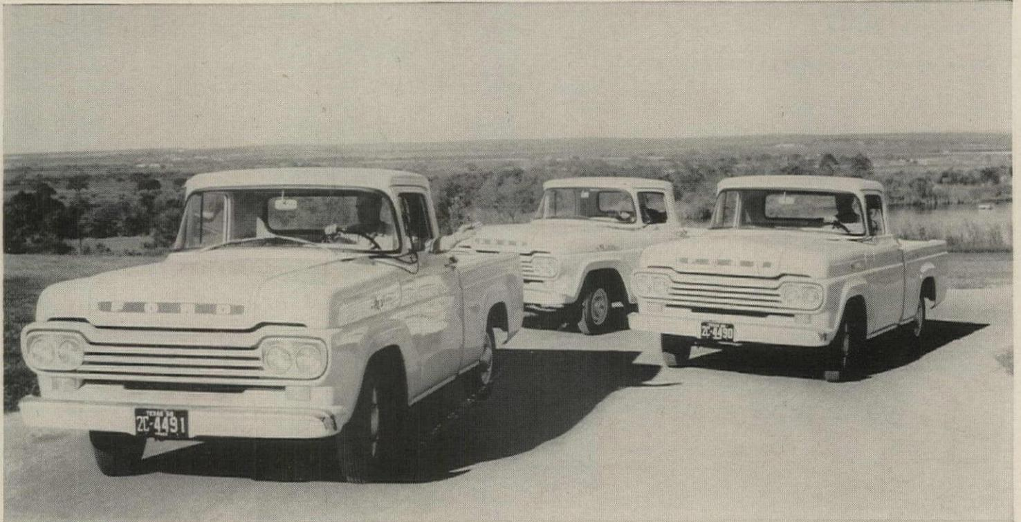
'59 Ford pickups running one of the Economy Showdown courses set up by the research engineers. Like all the new '59 pickups tested, these are regular stock models with a standard six-cylinder engine, 3-speed transmission and standard rear axle ratio.
