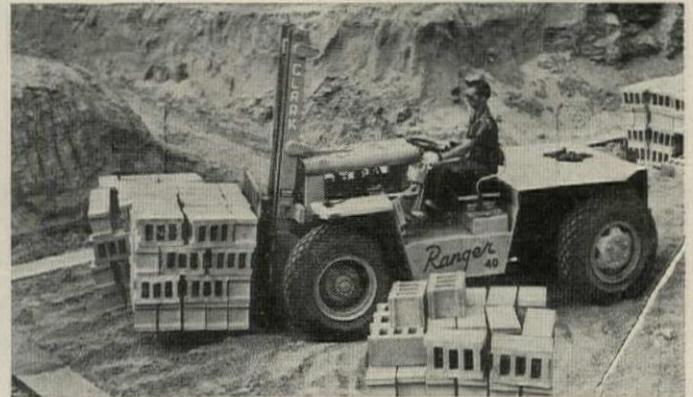
**Ranger fork trucks** to handle 4000 to 6000 lb loads have been introduced by Clark's Industrial Truck Div. Big wheels, oscillating axles, two and four wheel drive get the unit around rough building sites at speeds to 23 mph. Bi-angular steering turns Ranger in a 163" radius.
