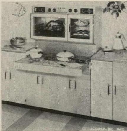
**Tappan 400 is now built-in.** This version gets two eye-level ovens, broiler, four burner tops, and double-blower fan into 40" of wall space (vent duct adjusts to stud space). Controls are safely above ovens; one 2600-w and three 1500-w burners are hidden under countertop when not in use. Fluorescent tube beneath ovens lights countertop. Retail price: \$695.
