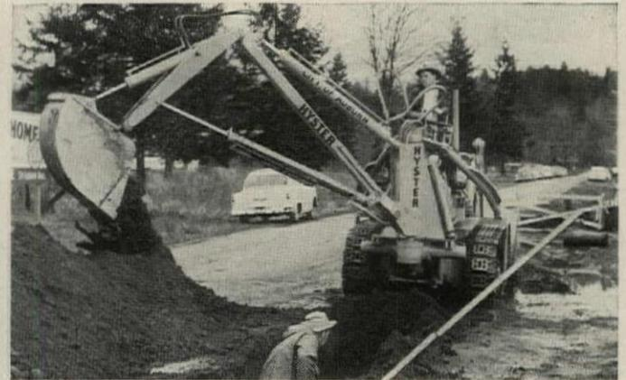
**Hyster** has a new hydraulic backhoe for use on Caterpillar D4 tractors or 955 Traxcavators. The unit will dig down 13', load to height of 9'7½". Full-power swing works through 240° arc. Buckets hold ½ cu yd, come in 13", 21", and 29" widths. Back stay struts oscillate with tracks.
