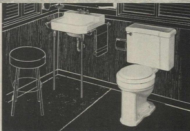
**Washdown Closet and Lavatory**, featuring No. 900 Washdown Unit Closet with 12-in. rough-in, lifetime nylon seat ballcock, two-bolt hitch and extended horn for quick installation. No. 310 Ledge-Type Lavatory, 19 by 17 in., is complete with No. 141 Centerset and has concealed overflow, integral soap dishes, anti-splash rim. In stainless white, or petal pink, wedgewood blue, forest green, driftwood tan, daffodil yellow, cloud gray.
