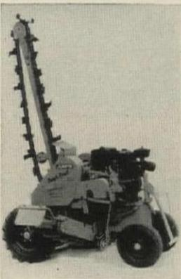
**Arps M-A Trench-Devil** is a medium-sized, self-propelled tool that will cut trenches 2¾", 3½", 4", 6", or 8" wide, up to 54" deep, and up to 1200' per hour. Hydraulic drive lets you change speed or direction on the go. Hydraulic boom raises and lowers chain. Reversible rubber belt conveyor can dump dirt left or right of trench. The M-A can travel over the road on its own power at 2¾ mph.
