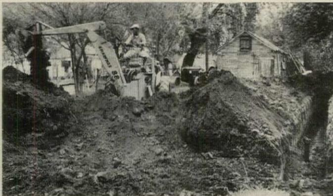
**Shawnee 88 backhoe** is a new high-speed digging tool. Two single-acting cylinders give uninterrupted 188° swing, keep chain under tension to prevent slop and compensate for wear. Bucket cylinder is hidden in the 88's bucket boom so it will not be damaged and cause job delays.
