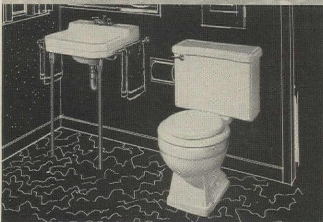
**Reverse Trap Closet and Lavatory**, featuring No. 1200 Reverse Trap Unit Closet. Vortex swirl-flush action, 12-in. rough-in, two-bolt hitch and extended horn for quick installation. No. 380 Ledge-Type Lavatory, 20 by 18 in., is complete with No. 143A pop-up and has concealed overflow, integral soap dishes, anti-splash rim. In stainless white, or petal pink, wedgewood blue, forest green, driftwood tan, daffodil yellow, cloud gray.
