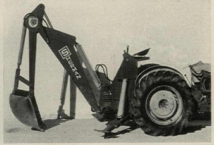
almost 20,000 lb. When swinging, drive elements are under tension and under positive control. In Ford installations the Panther has an electric-fan-cooled heat exchanger to keep unit working under extreme conditions.
