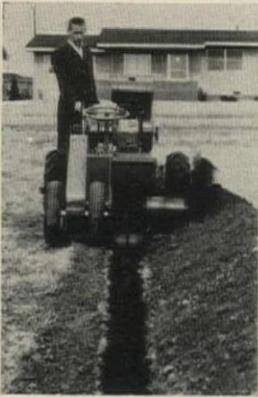
**Charles M-3 Ditch Witch** is made with optional digging teeth to cut 3", 4", 6", or 8" wide trenches. Its three-piece telescoping boom may be 2', 3', 4', or 5' long. Its three-piece chain has heat-treated teeth with Studite cutting edges, cuts to 2', 3', or 4' depths. Chain has spring tension adjustment to eliminate stalling. Power is supplied by 9.2-hp Wisconsin engine with Borg-Warner clutch reduction unit.
