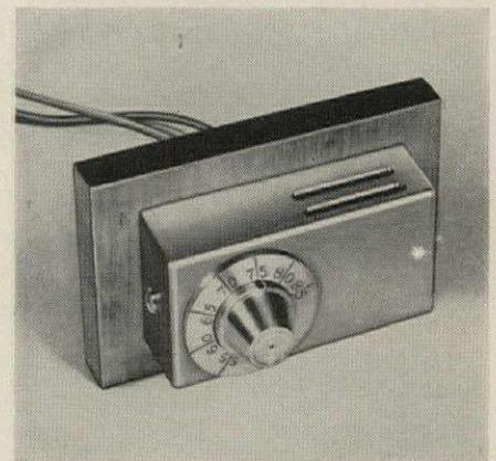
**Gas-heat modulator** is controlled by tiny thermistor which reacts immediately to small changes in temperature. Flame size is varied to maintain a steady ambient, eliminate off-and-on cycling. Usual thermostat acts as top-limit switch to cut off burner when atmospheric temperature rises above heating level. Blower operates continuously, prevents dead-air blankets. Price: \$82-\$94.
