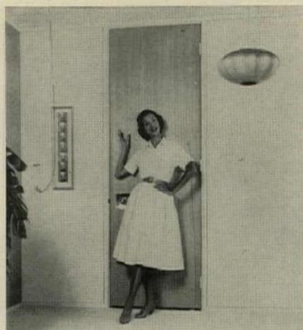
**Ceiling-high doors** that cut cost of overhead framing are now being made by Simpson Logging. Hollow-core flush doors are made 7'11" long and may be end-trimmed as much as 3" at the top to allow fitting. A 5½" lock rail extends the full width so lock can be set back as far as you wish. Doors are available in ribbon and rotary Lauan, rotary birch, and hard-board.
