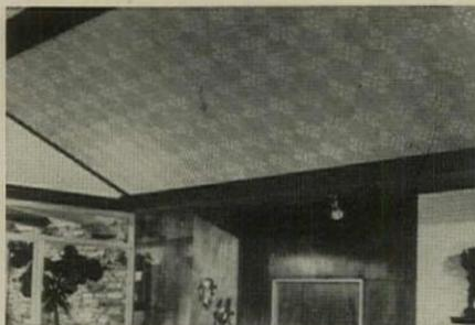
**Decorated silent ceiling** is new from Kaiser. Material is pinhole perforated Firtex on which a choice of six pastel colors have been printed. Ceilings come in all standard sizes with fir-lock or butt joints for stapling or gluing. Ceiling absorbs up to 70% of noise striking it manufacturer claims.
