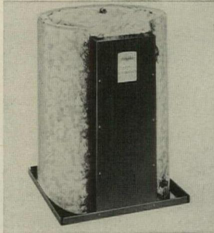
**Hide-away water heater** can be built into dead corner space in cabinets and save long pipe runs. Tank is extra-heavy gauge galvanized steel, tested to over 300 psi. Extra thick insulation will keep water hot three days. Calrod units come in various wattages for 236-v systems. Heaters fit in 24" x 24" space, 26<sup>3</sup>/<sub>4</sub>" high for 30 gal unit, 54 7/16" for 40 gal. Ten-year protection plan.
