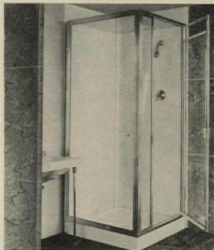
**Prefabricated shower** is entirely self-contained. Drainpan is pre-cast terrazzo. Sandwich walls have Formica interior faces, foamed styrene insulation and stiffening, steel exterior shell, eliminate need for ceramic walls and floor; give long-lasting, low-maintenance surface. Styrene foam cuts sound transmission. Glass panels are factory glazed in anodized aluminum.
