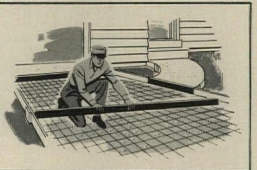
**FLEXCELL\* EXPANSION JOINT.** Asphalt impregnated fiber board. Non-extruding, resilient. Pre-cut strips. For use wherever concrete meets concrete. Also for perimeter insulation of slabs at grade; sill sealer; plate sealer. Variety of thicknesses.
