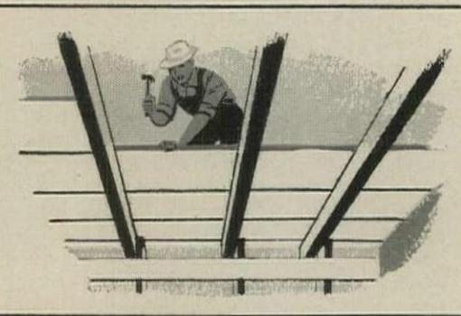
**INSULATING ROOF SLABS.** Roof deck, insulation, built-in vapor barrier, finished ceiling, plus continuous vapor seal at all joints. (Or without vapor seal and barrier.) Ideal for exposed-beam construction.
