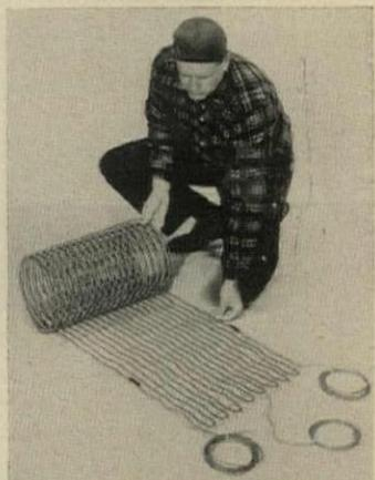
**Easy-Heat Sno-Melter** is designed to work at 42 watts per sq ft. The 18"-wide mesh is galvanized steel; the interwoven resistance wire is thermoplastic insulated. Wire mesh prevents burn-outs during concrete pour, gives some reinforcement to paving. Stock mats are 10' long. Non-heating leads and ground are attached.
