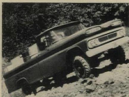
**4x4 PICKUP** in three wheelbases and 1/2 and 3/4 ton ratings, has full floating axles.
