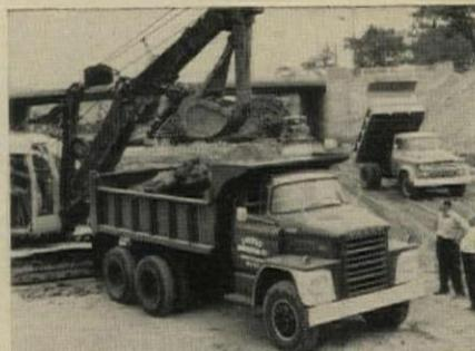
**CAB-FORWARD CT800**, a 45,000-lb gvw model, has swing fenders for easy access.
