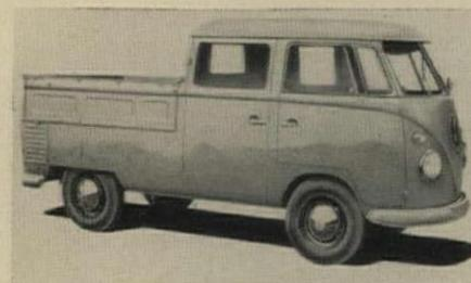
**Double-cab pickup** is latest version of the VW truck. Cab seats six as work crew carrier. Rear seat can be removed to give 63 cu ft of enclosed lockable space. Sides of 32-sq ft rear deck drop so it can be loaded from all sides. Body mounts on standard VW chassis. Price on east coast: \$2,150.
