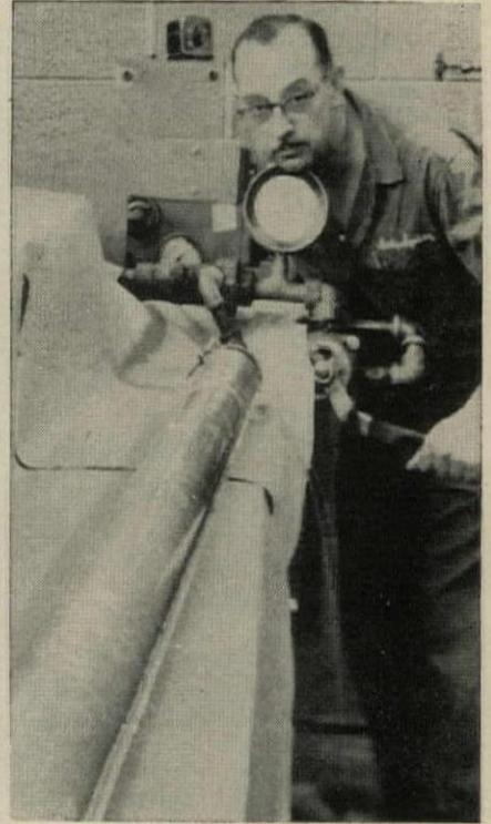
**FINISHED ROUND DUCT** has flat bead on either side where thin metal walls join.
