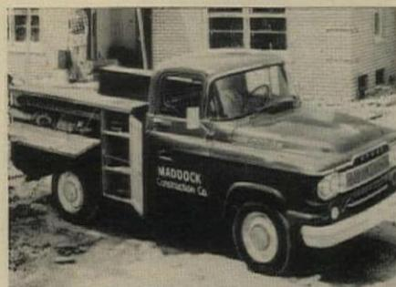
**D 200 TRADESMAN** has 116" wheelbase, can have a 120-hp six or 200-hp V-8 engine.
