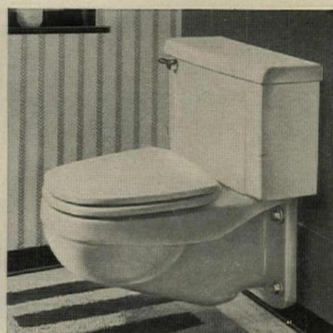
**New wall-hung Norwall toilet** hangs on sturdy cast iron combination carrier. Installs easily on standard 6" stud wall. Since it is completely off the floor, it makes fixture and floor cleaning easy, fast. Seat and cover snap off for thorough cleaning.
