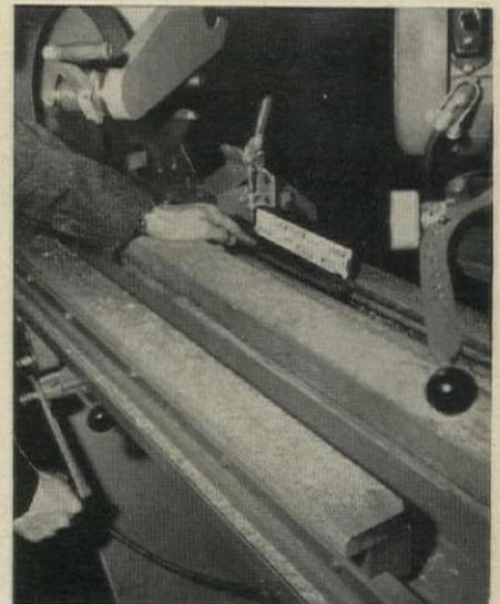
**SPAN AND PITCH** of truss are set on this indicator panel by rotating a front-mounted crank. This sets angle and depth of cut.
