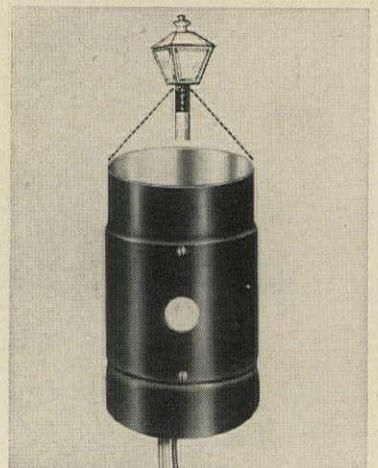
**Post lantern switch** turns yard lights on and off at dusk and dawn. Time-delay photoelectric eye activates switch, allows three-minute lag so lights will not be turned off accidentally by car headlights. Unit is compact, prewired, will fit any 3" post. Switch works on 115v with 400-w capacity. Temperature compensator will withstand -25F to 150F.
