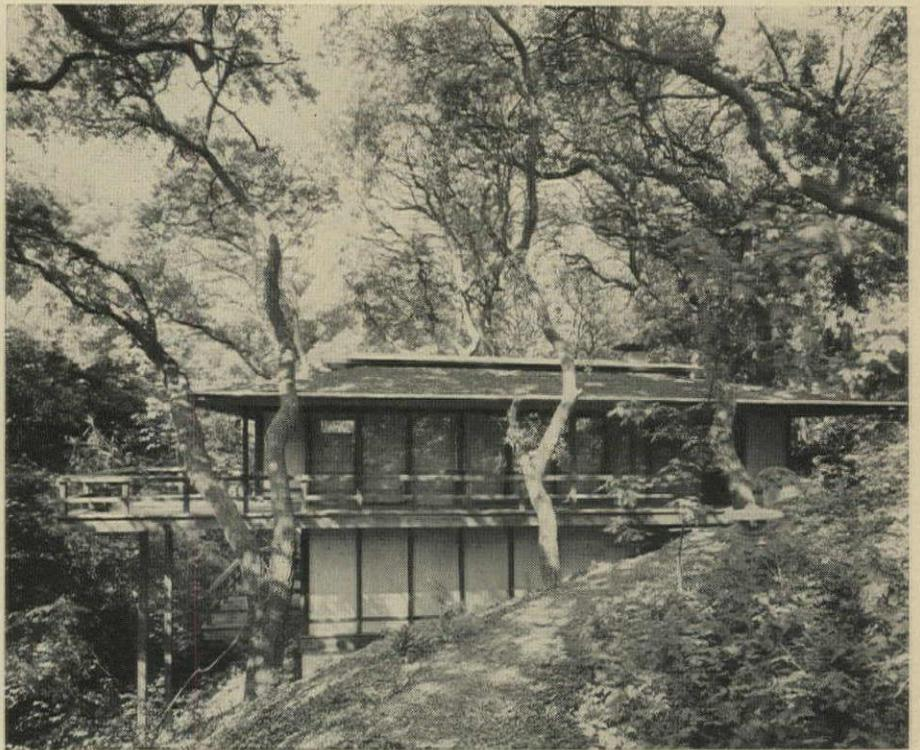
**TWO-STORY PANEL** effect comes from joints of asbestos-cement panels matched to joints of glass panels above in this California house. Architect: Charles Warren Callister. →
