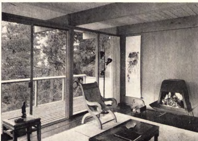
Living room opens to one of three balconies. Wall is prefinished luaun plywood; floors and ceilings are 2x6 t&g; balconies are 2x4s, 4" oc.
