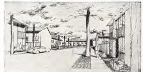
ALTERNATE SCHEME for same number (280) of families replaces uniform twin houses with groups of varying lengths and setbacks in a street pattern excluding through traffic.
