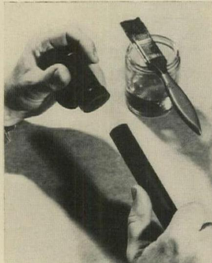
**PIPE ASSEMBLY** is simple: brush on solvent, slip pipe into fitting, let joint set.
