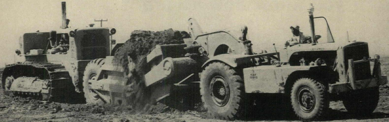
**TWO-WHEEL SCRAPER**, pulled by one tractor, is pushed by another to speed job. Scrapers dig, carry, and spread dirt in one working cycle.
