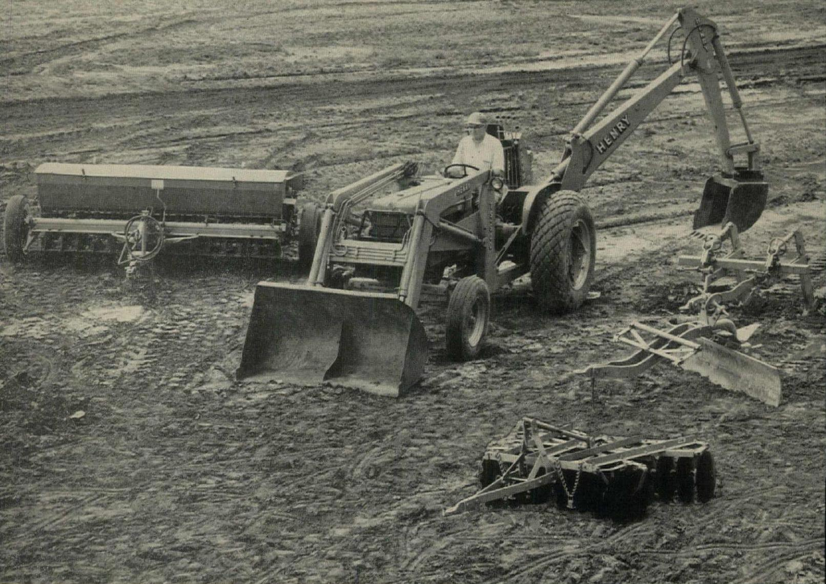
UTILITY TRACTOR with front loader and backhoe also takes other attachments.\* Photo taken for H&H at Allis-Chalmers proving grounds.
