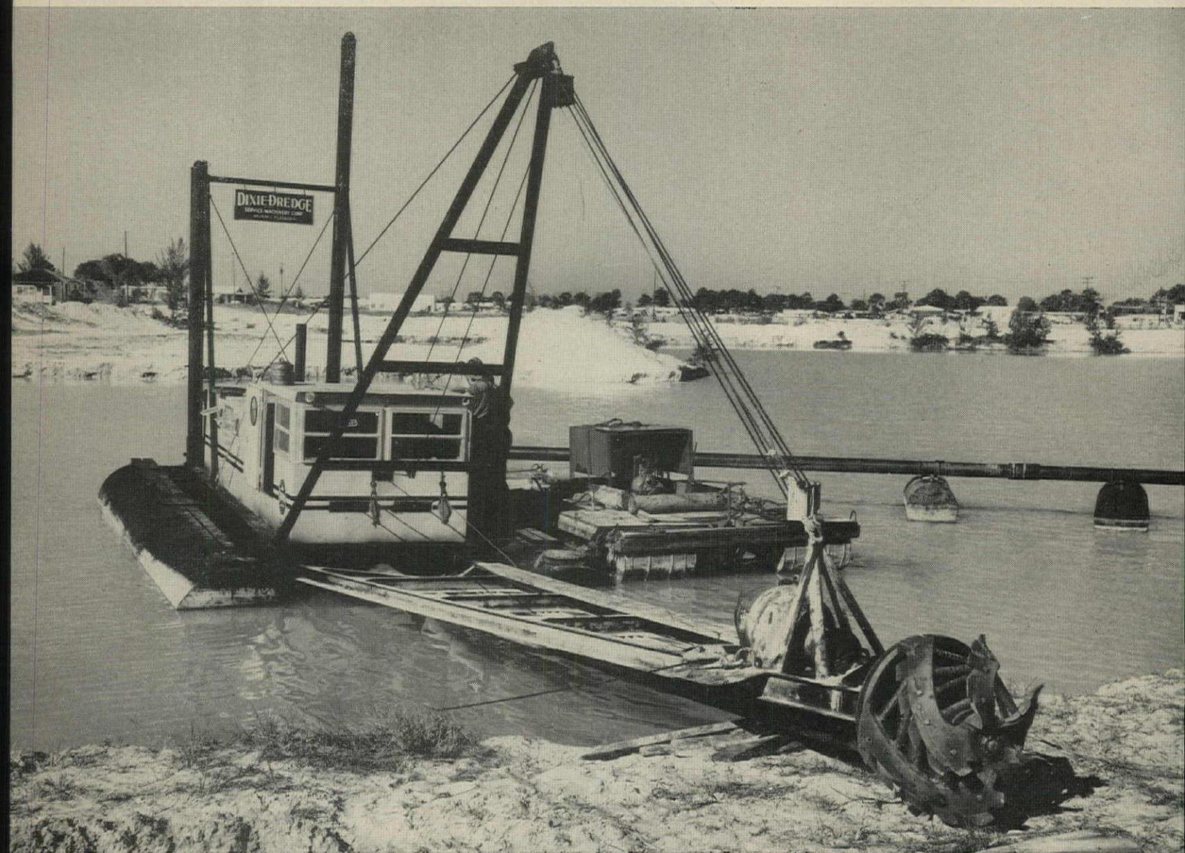
**SMALL DREDGE** dislodges and sucks up underwater soil with cutter head, foreground, and pumps it through tailpipe, right, to reclaimed site.
