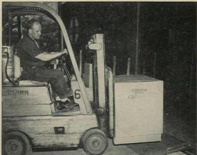
**PALLETIZED LOADS** for ready handling in transit and in stock are possible with the new standardized parts, can save 75% in storage space.
