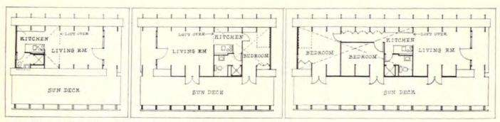
THREE TYPICAL PLANS show flexibility of system. Model at right has over 1,000 sq ft of living space, including second-level sleeping loft.
