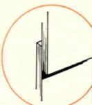
Fastener cannot be seen <u>after</u> overlapping panel is applied.
