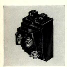
New Duplex Pushmatic puts two circuits in the space of one single breaker. Gives: identical, independent coil-magnetic protection in each pole of all Duplex breakers; positive one-bolt connection; pushbutton convenience.
