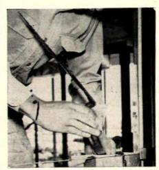
Layout tape for brick masonry is claimed to cut layout costs up to 50%. Tape is marked for course height and bond layout for brick to be used, self-adheres to corner pole, sheathing, etc to mark spacing. Brik-Hite tapes come in eight markings, cover most brick sizes being made.
