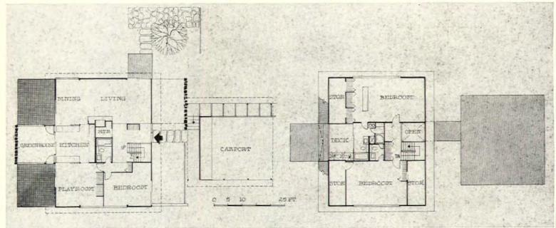
FLOOR PLAN provides 2,000 sq ft of living area on two floors. Mechanical core runs up through center of house. Note sun deck off upstairs bath.
