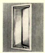
Self-storing screens are planned for use with casement and awning windows. Screen-O-Matic screens are held in place with rigid vinyl channels. Fiberglass screening rolls into aluminum roller housing. Bottom rail is a heavy aluminum extrusion, rubber sealed, and locked in place with nylon catches.
