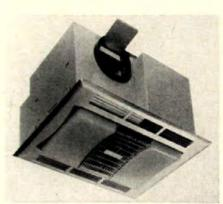
Electric heating for bathrooms and kitchens is supplied by new Westinghouse units. The heater-light-fan shown has a 1,200-w heating element, two 60-w lamps, and a 175-cfm blower separately controlled at the wall. Unit also comes as a heaterlight or a 1,000-w heater only. All mount flush between ceiling joists.
