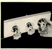
Two-piece escutcheon of Speakman's new Kent fittings simplifies installation of wall valves on uneven surfaces. Wall flange can move up to 1" to adjust to variations in rough-in or wall thickness. Once in place, flange is made fast to the valve sleeve with a set screw.
