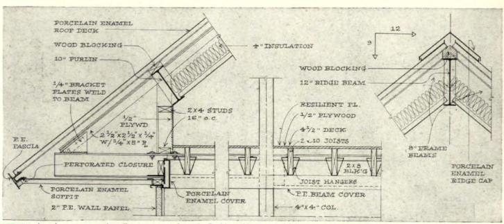
DETAILS show how trusses and purlins support roof panels. Decking without porcelainized enamel is standard in commercial concrete construction.
