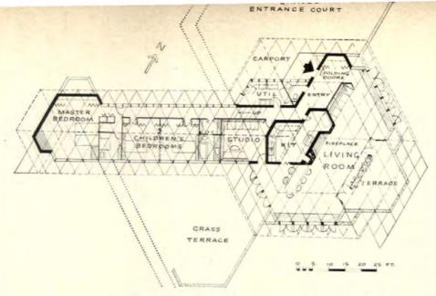
Diamond-shaped module determines plan of most rooms. Sides of the diamond-shape are 4' long, its interior angles are 60° and 120°. Wright used such nonrectangular modules to create more fluid and less boxlike spaces. In this house, the module was abandoned in the bedroom wing.
