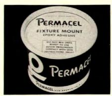
Fixture adhesive provides a new way to hang hooks, brackets, lighting receptacles, furring strips, electrical fixtures, towel and cup dispensers, nameplates, signs, etc. Adhesive will bond to wood, tile, glass, metal, plaster, concrete, drywall, etc. Only five- to ten-second pressure is needed. Two-component epoxy comes in an 8-oz cup holding equal parts of resin and hardener.
