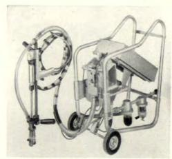
powasert nailer is air-operated at 95 to 120 psi, draws 14 to 17 cu ft per minute. Model shown drives nails 2½" to 5" long at 50 to 75 per minute rate. Hopper holds 8 lb of nails. Hose gives 12½' working radius. Gun weighs 16 lb, separator 60 lb. Smaller models weigh 7 lb, handle nails 1¾" to 3½" long at 50 per minute rate over a 25' radius. Prices: \$1,295 to \$1,445.
