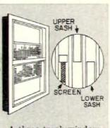
A three-track window has separate guide paths for each insert, is thus self-storing.
