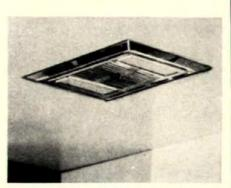
New ceiling unit by Trade-Wind combines heat, light, and ventilation. Reversible axial-flow fan adds forced-air heating to radiant heat from resistance coil, also acts as exhaust fan. Unit comes in five other versions: 1) heater alone, 2) lights alone, 3) light and heater, 4) exhaust only, 5) exhaust and lights. Control is wall switch.
