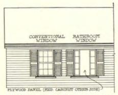
BATHROOM FENESTRATION. "We didn't want the master bathroom window (right) to break the fenestration pattern of the house but we didn't want a full-size window in the bath. So we built a medicine cabinet between two narrow windows, backed it with a piece of plywood on the outside, put shutters on either side.
