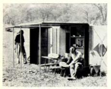
FULLY OPEN, unit forms semi-circular shelter. Side flaps of trailer forms porch roof.
