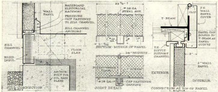
DETAILS of sandwich panel connections show how bottom edge clips to sill, how interior panel joint is gasketed, how panel top grips head bracket.
