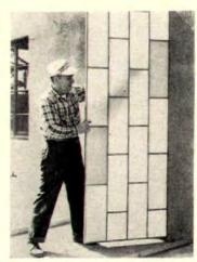
Translucent walls are possible with Seaporcel's new units. Panel consists of two fiberglass-reinforced acrylic-polyester sheets laminated to an extruded aluminum grid. Panels are lightweight (11/2 lb a sq ft) but strong (resist impact of 2,000 psi). Colors cut glare, add decoration. Panels come in sizes to 4'x20', in various types for walls, partitions, skylights, canopies, entranceways, etc.
