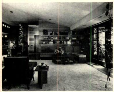
Sitting area at east end of living room is built in as is most other furniture. Bench is placed so as to offer a view of the landscape as well as the fireplace. Partitions are of horizontal boards and battens, nailed to a 34" plywood core.
