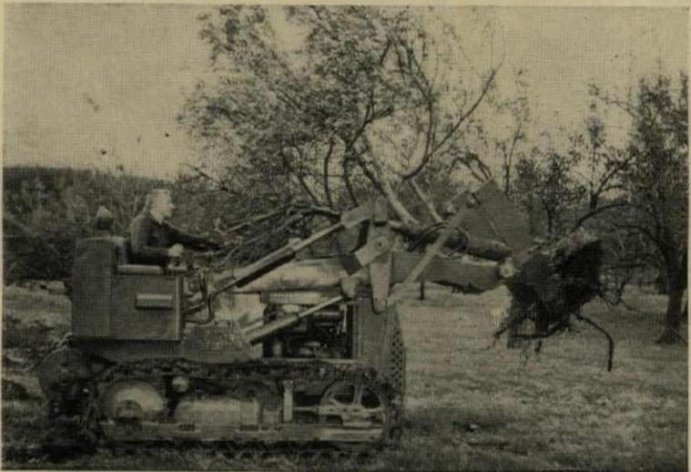
3. **SMALL TREE DIGGER** on tractor can move 4" tree in 30 seconds.
