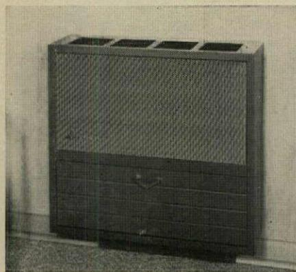
**Coleman** now offers a through-the-wall gas heater with a sealed combustion chamber. Two models give 22,000 and 30,000 Btuh from case 30"x26"x9". Unit fastens to studs 4¾" above floor. Outside air is used for combustion and exhaust vents directly to outdoors. Options include manual, automatic, or remote controls, two-speed blower, vent extension for thick walls, decorative insert panels.
