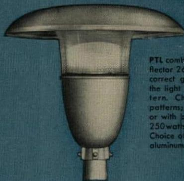
PTL combines rigid spun-aluminum reflector 26" in diameter with optically correct glass refractor which directs the light downward in an even pattern. Choice of seven IES light patterns; lamps up to 10,000 lumens, or with ballast for mercury lamps to 250 watts. Available with photocontrol. Choice of six pastel colors or natural aluminum. For 3" or 7" post.
