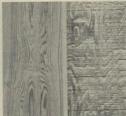
**Satin-finish redwood** is factory-coated with a clear high-solids lacquer that allows the wood grain to show through. Reverse side, right, is rough sawn. Paneling is being made in 3/8" through 3/4" thicknesses in various widths. Panels are protective wrapped.
