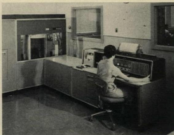
**Special electronic computer** is called a "random access memory" unit. Information is filed on discs in "juke box" unit, left. Any fact can be found within two seconds.
