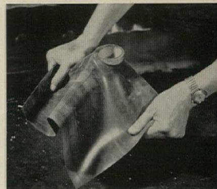
**Pre-cut flashing** for standard vent stacks is now being packaged by Dow. The sheets are made of Saraloy 400, a flexible and elastic plastic. Sheets are nominally 1/16" thick, come 18" x 18" and 20" x 20", with holes for 2½", 3", 3½", and 4" pipe. Pieces are packed 12 to a box. The product is FHA accepted.
