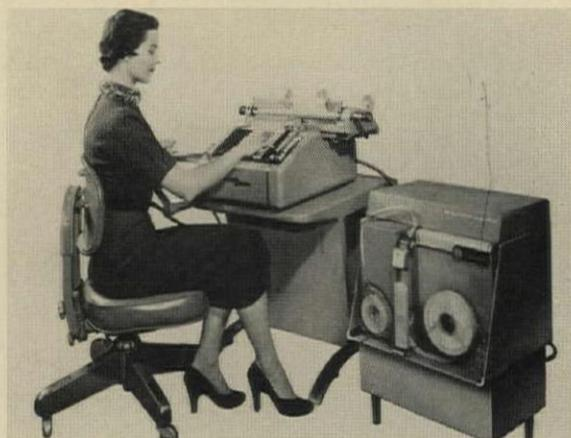
**Tape punch unit** produces a perforated tape for use in electronic computers. This unit takes data directly from a bookkeeping machine and turns it into machine language.
