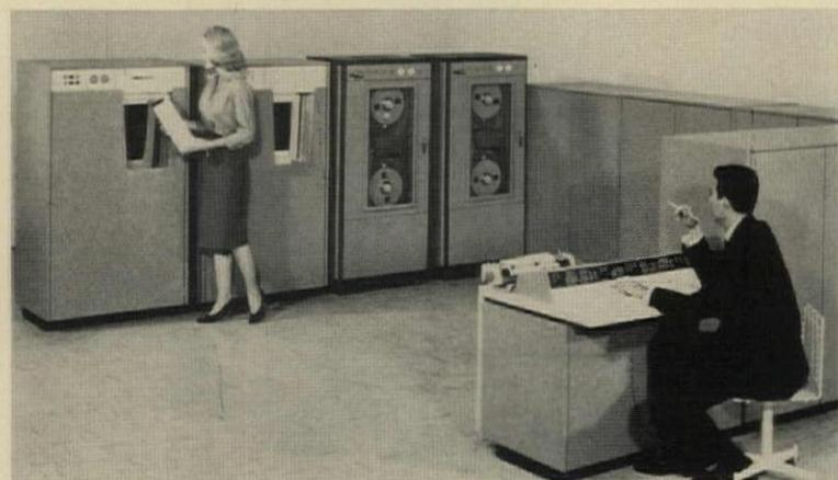
**Big electronic computer** operates either from magnetic tape (in real units, center), or from magnetic cards (in units at left) which are high-speed versions of punched cards that can be "read" at a rate of 150,000 digits per second. At right is the computer's control console.
