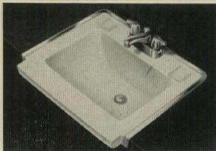
**Countertop lavatory** has an exposed front, fits a standard U-shaped clamp-down frame. The vitreous china unit has two cast-in soap depressions, anti-splash rim, concealed front overflow. It takes a standard 4" centerset faucet. Overall dimensions are 18" x 20", basin is 15" x 7" x 7". Colors are compatible with most current bathroom fixtures.
