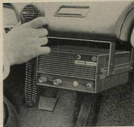
**New two-way radio** designed to work in the 27 to 50 mc and 150 to 174 mc bands is the most compact offered by GE. Pacer model is 15-w unit with 15 tubes, two transistors, draws only 4.2 amp so as not to overload the car battery. Special generators and heavy-duty batteries are not needed. The entire unit occupies a space only 4¼" x 7¾" x 13½", weighs only 10 lb, is smaller than even transistorized models.
