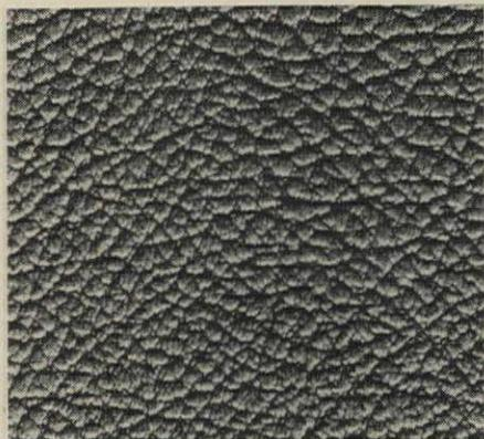
**Morocco-grained paneling** copies the look and texture of fine leather in an otherwise unfinished tempered domestic hardboard. The makers suggest various painting techniques can create interesting effects. Panels are made 1/8" and 1/4" thick in usual sheet sizes.
