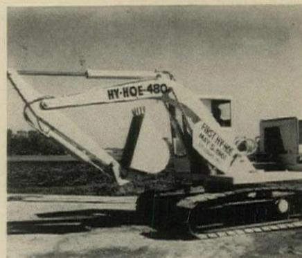
**New crawler backhoe** has the highest flotation available—3 psi on 24" pads—the maker claims. A three-pump hydraulic system lets the operator work boom and bucket while swinging. Double-acting cylinders are powered at 1,500 psi. Model 480 can dig 150', 5' to 6' deep, in one hour. Unit has 23' reach, 15' digging depth.
