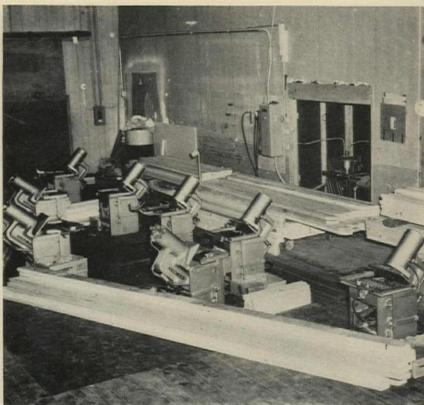
**This machine assembles trusses at a 240-a-day rate**
