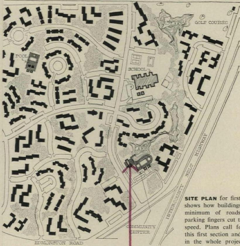
**SITE PLAN** for first 195-acre section shows how buildings are laid out. A minimum of roads and cul-de-sac parking fingers cut traffic—and traffic speed. Plans call for 2,751 units in this first section and a total of 5,000 in the whole project.
