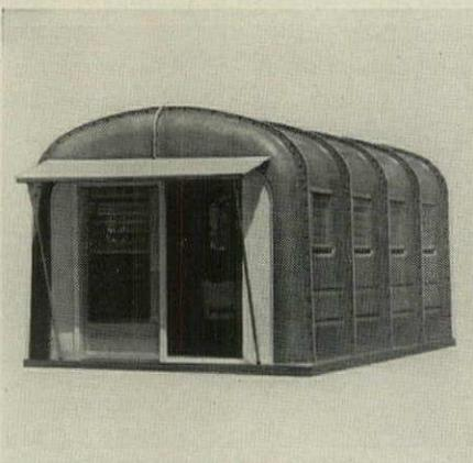
**Reinforced plastic building** is made up of sections bolted together on site. Assembled building is 10' wide, 8' high, and can be made of any number of 4' sections. It can be used as a temporary field office or as a permanent structure. Unit is designed to withstand 35-lb snow load and 100-mph winds and is offered in a variety of molded-in colors.
