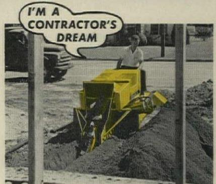
THE T-78 has ground-gripping (track) traction, high flotation (3.6 lbs. psi ground pressure), and is only 37" wide. Spoil can be delivered to left or right. Trenches up to 840 feet per hour.
