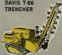
Digs where others can't because of its compact design, ground-gripping traction and high flotation. Trenches from 18" wide to 24" deep, to 4" wide, 66" deep.
