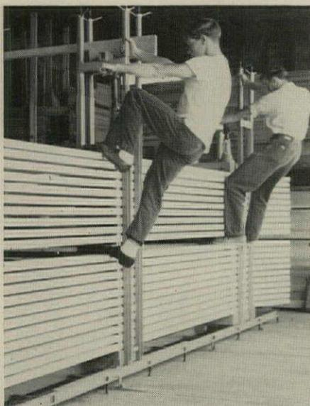
**BELL JACKS** apply pressure to load-spreader plates over each gusset location.
