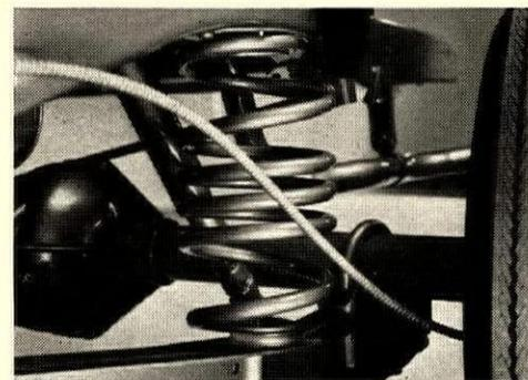
At rear, new variable-rate coil spring suspension.
