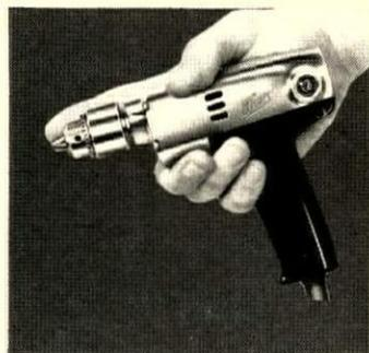
**Compact ¼" electric drill** is 6½" long, 2" at widest part, weighs 27 oz., runs at 1,250 rpm on 115-volt a.c. Diode converts input to d.c. and permits compact d.c. motor which supplies full power. List price: \$32.50. Thor Power Tool, Aurora, Ill.
