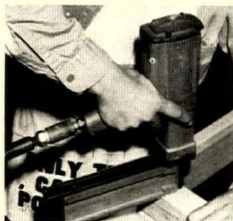
**Heavy-duty nailer** for cabinets, windows, doors, etc. will drive and countersink special Speedfast corrugated fasteners at a rate of 80 per min. Can be converted to drive other special fasteners. Retail for \$185. Speedfast, Long Island City, N.Y.
