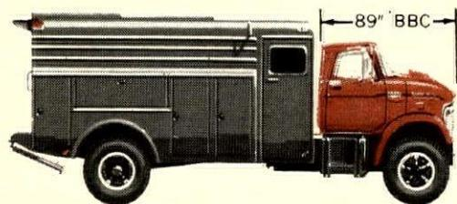
**FORD'S NEW SHORT-BBC CONVENTIONALS**—Ford's N-Series trucks measure only 89 inches from bumper to back of cab. Short wheelbase, wide-track front axle, and narrow front fender width provide superior maneuverability. You get a much smaller turning radius than with long-BBC conventionals—even shorter than with most trucks with similar BBC's. Ford's short-BBC design lets you use 1-foot longer bodies within the short overall length that's essential for city work.
