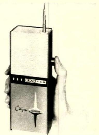
**Pocket-size walkie talkie** has 1 1/2-mile range in average areas, more where area is flat and open. Push-to-talk switch also provides volume control. Rechargeable battery gives about eight hours of intermittent operation per charge and lasts about 2,500 hours. Radios come with batteries and charger, cost \$60 a pair in kit form, \$80 a pair completely assembled. EICO Electric Instrument, Long Island City, N.Y.
