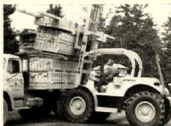
**Medium-capacity fork lift** handles up to 12,000 lbs, has four-wheel drive designed for job-site lumber handling. It can tow loaded trailers, or can itself be towed to the site with drive disengaged. Hyster Co., Portland, Ore.
