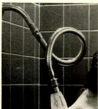
**Flexible shower tube** lets shower head be raised a foot above or below its normal position, locks itself in place. End fitting attaches to standard-size shower-outlet pipe. Mueller Brass Co., Port Huron, Mich.
