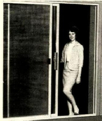
**Rogers** aluminum sliding door can be converted from right- to left-hand opening. Changeover can be accomplished in less than an hour by turning glass panels upside down. Rogers Industries, Inc., Jackson, Mich.
