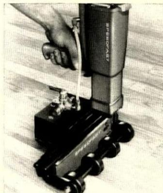
**Automatic stapler** has attachment which spaces staples and fires fastenings as tool is rolled along surface. Spacing can be from 2" to 8". Gun uses staples or nails from ⅝" to 2". Speed-fast Corp., Long Island City. For details, check No. 171 on p 219
