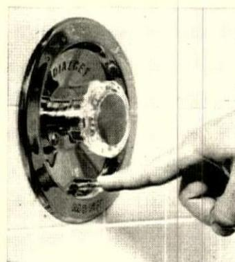
**Diverter valve** for changing tub flow to shower flow has been added to the "Dialcet" single-handle unit. A push-button below the valve handle is pressed to start the shower flow. Moen Faucet, Bellwood, Ill.
