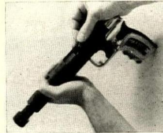
**Piston-type gun** drives fastenings into work at low velocity. Blank cartridge drives the piston which in turn sets the fastener. Unit weighs 4½ lbs. Winchester-Western Div., Olin Mathieson Chemical Corp., New York City. For details, check No. 170 on p 219
