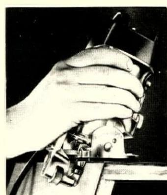
**Veneer trimmer** has swivel base which swings 45° in either direction, permits edge beveling of angled joints. Tool also scribes work and cuts it in a single operation. Stanley Works, New Britain, Conn. For details, check No. 173 on p 219
