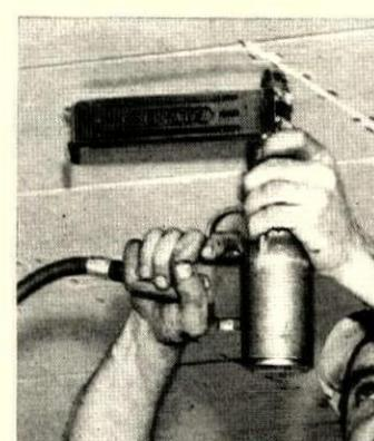
**Power stapler** is available in models that handle staples from ⅜" to 2", and T-nails from 1¼" to 2½". It operates on air pressures as high as 90 psi or as low as 40 psi. Bostitch-Calwire, East Greenwich, R. I. For details, check No. 174 on p 219
