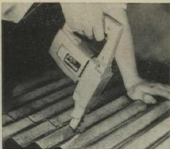
**Power nibbler** makes straight, curved, pattern, and pocket (inside) cuts from a 1/2" diameter starting hole in sheet and corrugated metals. It cuts 40" of 18-gauge steel per minute, weighs 5 1/4 lb., and lists for \$64.95. Skil Corp., Chicago. For details, check No. 13 on p. 182
