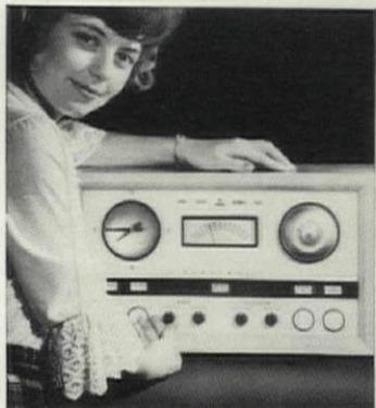
**Electric control center** for motel units operates lights and TV, adjusts room temperature, and checks outdoor temperature. It can be mounted on a bedside table or in a headboard. Minneapolis-Honeywell, Minneapolis. For details, check No. 4 on p. 182
