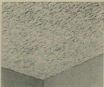
**Acoustical tile** has a textured surface that conceals joints, absorbs up to 90% of noise reaching it and reflects more than 70% of light striking it. Acoustone Glacier comes in 12"x12" and 12"x 24" tile with plain or foil backing. U.S. Gypsum, Chicago.
