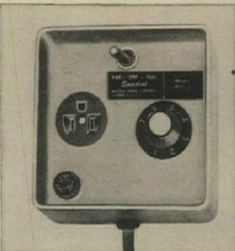
**Motor speed control** regulates speed of any electric tool. By turning a knob, Speedial provides high speed (for cutting or drilling plastic), medium speed (wood), low speed (masonry), or very low speed (steel). Lutron Electronics, Emamus, Pa. For details, check No. 10 on p. 182
