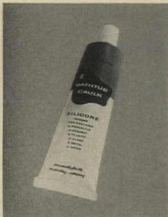
**Bath caulking** is applied from a squeeze tube with a special nozzle to give various sizes of bead. Silicone rubber caulk dries in 1 hour, cures in 24 hours, but stays flexible to accommodate swelling and shrinking. Dow Corning, Midland, Mich.
