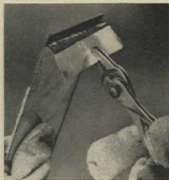
**One-part adhesive** is used for bonding panel skins and cores and for bonding laminates to countertops. Bondmaster G442 retains flexibility, can be roll-coated or sprayed, requires high-temperature drying. Pittsburgh Plate Glass, Bloomfield, N. J.
