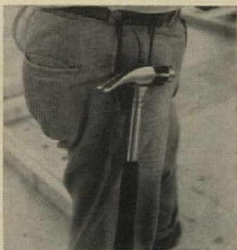
**Hammer holster** will end torn pockets and broken coverall loops. It can be hooked over a belt or looped on the ties of a nail apron. The holster is made of heavy wire coated with plastic to prevent rusting and scratching. Weyerhaeuser, Tacoma.
