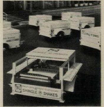
**Shingle-forming machine**, mounted in a trailer, produces aluminum roof or siding shakes at the site. Aluminum blanks are 3'x1', come in three textured patterns with natural aluminum or baked-enamel finish. Reynolds Metals, Richmond, Va.
