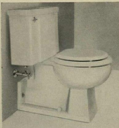
**Rear-discharge, floor-mounted toilet** is designed for slab construction in houses and apartments. Barlow's outlet is 4" above the floor so it is roughed in above the slab. Available in white and six pastels. Kohler, Kohler, Wis. (For details, check coupon No. 13 on p. 198)
