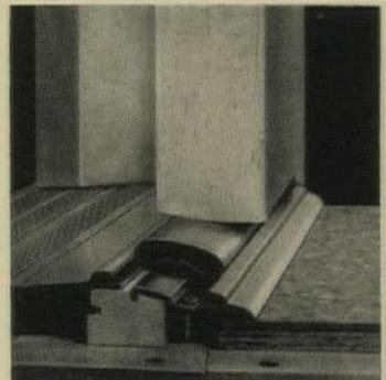
**Adjustable door frame** fastens directly to subfloor, has tilting saddle to fit any thickness of finished flooring from 3/8" (bottom) to 3/4" (top). Aluminum parts are separated by a wood thermal barrier. Rock Island Millwork, Rock Island, Ill. (For details, check No. 21 on p. 203)
