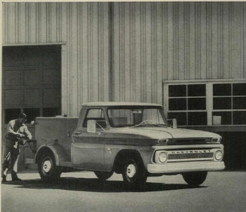
↑ **Chassis cab with special utility body** provides a handy repair shop on wheels. You can choose from five Chevrolet light-duty chassis-cab models in a wide range of wheelbases; get one that's just right for your special body. All feature 34-inch-width frames and independent front suspension.
